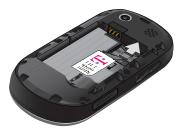
Note: If the card is not inserted correctly, the phone will not detect the SIM card. Remove the battery and re-orient the card back into the slot.
