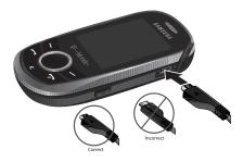
Note: The previous illustration displays the incorrect method for connecting the charger. If attempted, damage to the accessory port will occur therefore voiding the phone's warranty.
