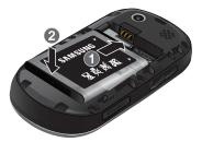
Reinstall the battery cover by sliding it back onto the phone until you hear it securely click. Make sure the battery is properly installed before switching on the phone.
