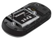
Carefully slide the SIM card into the SIM card socket until the card locks into place. Make sure that the card's
