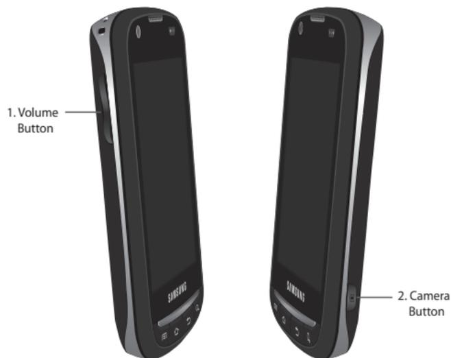
1. **Volume Button** adjusts the ringer volume in standby mode, the voice volume during a call, and media playback volume.
