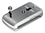
• To remove the battery, pull the top of the battery away from the phone (1) and disconnect it (2).
