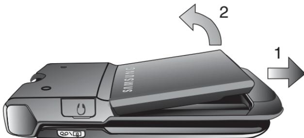
2. Grip the battery at the bottom and pull up and out at a 45° angle.
