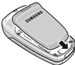
5. Press the battery down until it clicks into place. Make sure that the battery is properly installed before switching on the phone.
