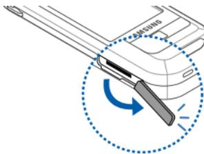
2. Plug the small end of the travel adapter into the device.
