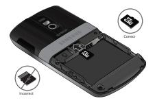
Warning!: The following illustration is the incorrect method for inserting the microSD card. If attempted, damage to the accessory port occurs therefore voiding the phone's warranty.
