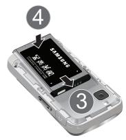
Replace the cover by lining up the tabs and then firmly sliding the cover away from the lens until it snaps into place.
