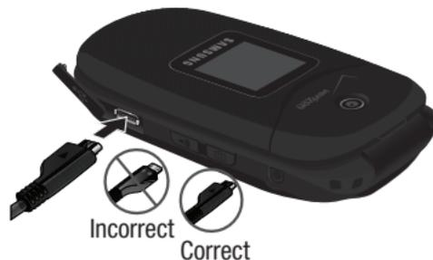
3. Insert the USB cable into the port.
