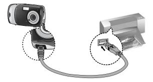
If you selected [COMPUTER] in Step 5, when you connect the camera to your printer, the camera status lamp(Green) will illuminate and the connection will not be established. In this case, disconnect the USB cable, and then follow the procedure from Step 2 and onward.
