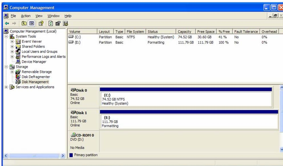
15. You will return automatically to the “Disk Management” window and will see the newly formatted Rocstor disk on the screen with the name you selected. If no new name was entered in the “Volume label,” the Rocstor drive will show up as “New Volume.” To rename the volume at this time, right click “New Volume” and click “Properties.” You can now change the volume name up to 11 characters. Click OK.
