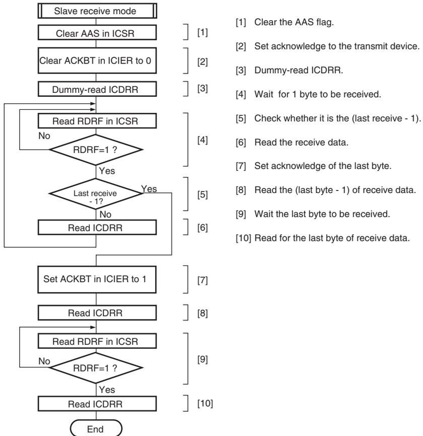
Supplementary explanation: When one byte is received, steps [2] to [6] are skipped after step [1], before jumping to step [7]. The step [8] is dummy-read in ICDRR.
