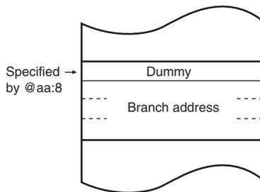
**Figure 2.8 Branch Address Specification in Memory Indirect Mode**
