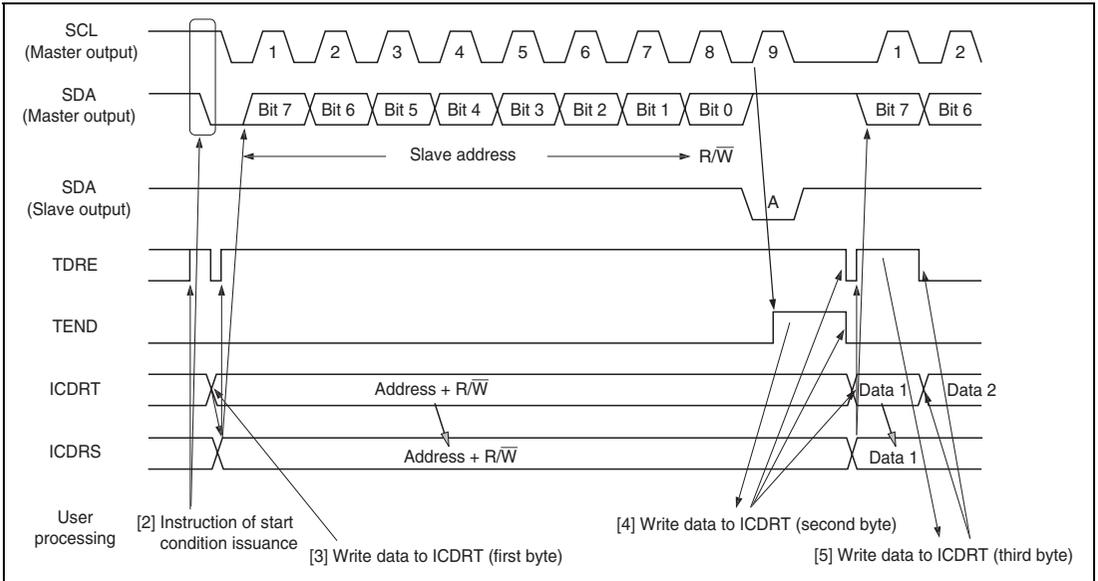
**Figure 17.5 Master Transmit Mode Operation Timing (1)**
