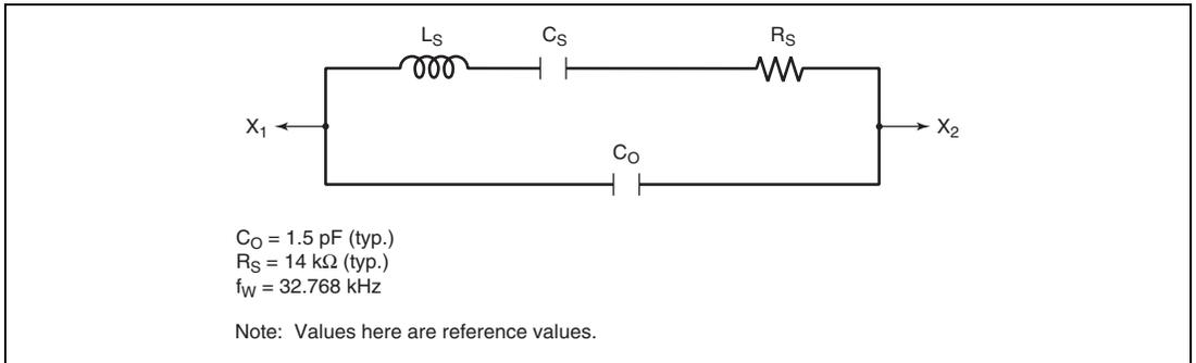
**Figure 5.17 Equivalent Circuit of 32.768-kHz Crystal Resonator**
