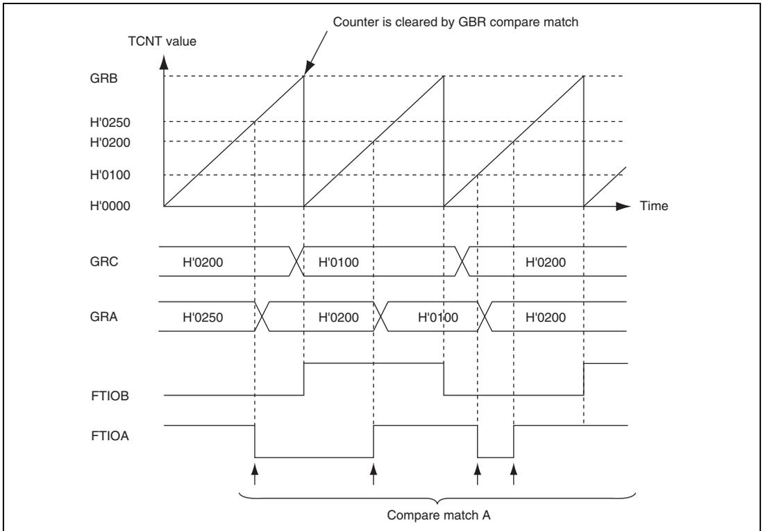
**Figure 13.38 Example of Buffer Operation (1)
