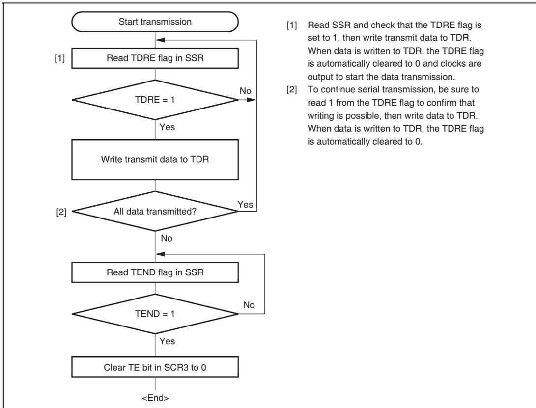
**Figure 16.11 Sample Serial Transmission Flowchart (Clock Synchronous Mode)**
