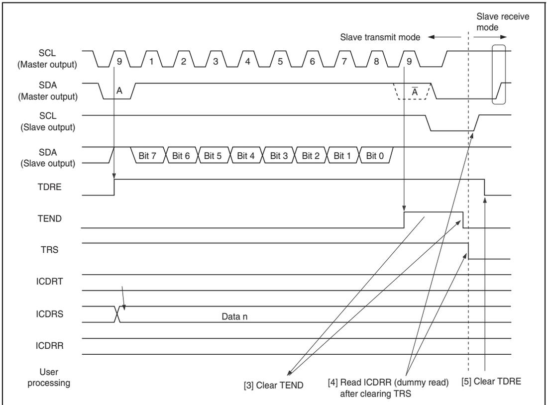
**Figure 17.10 Slave Transmit Mode Operation Timing (2)**
