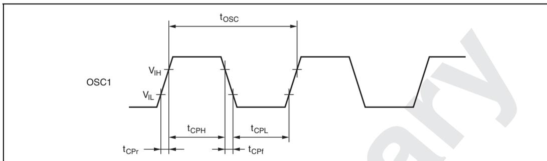
Figure 22.1 System Clock Input Timing
