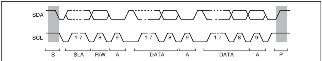
**Figure 17.4 I<sup>2</sup>C Bus Timing**
