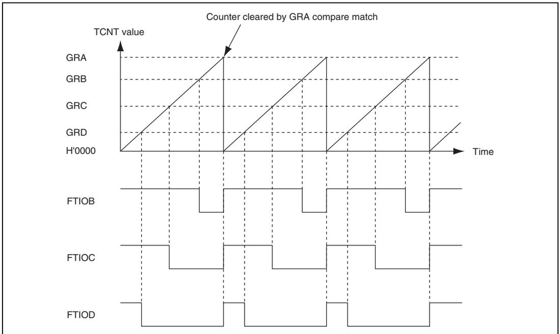
**Figure 13.22 Example of PWM Mode Operation (1)**
