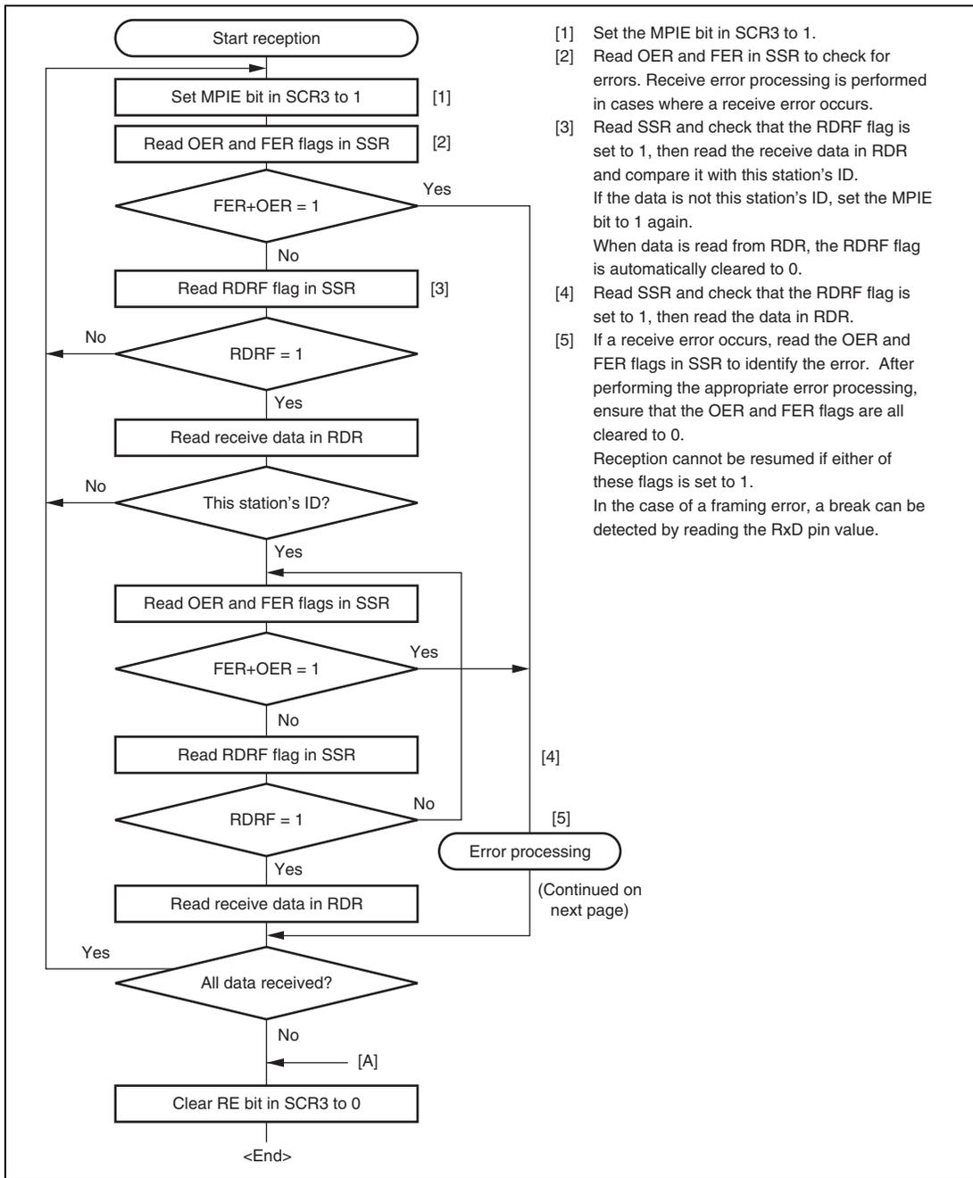
**Figure 16.17 Sample Multiprocessor Serial Reception Flowchart (1)**
