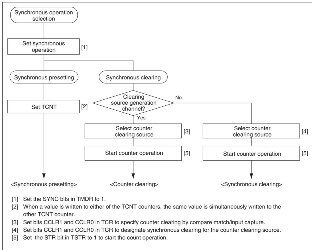
**Figure 13.19 Example of Synchronous Operation Setting Procedure**
