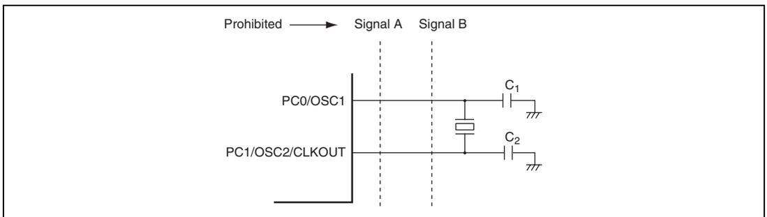
**Figure 5.19 Example of Incorrect Board Design**
