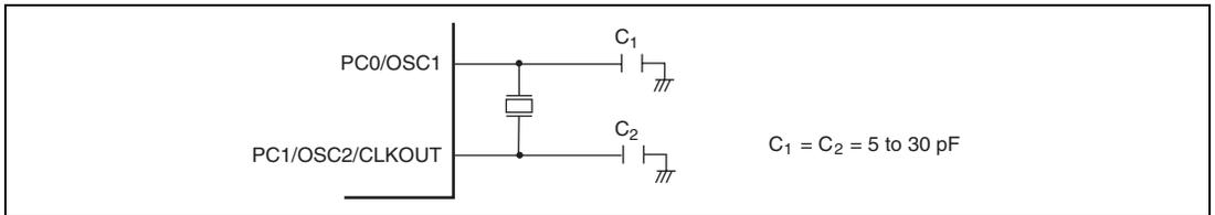
**Figure 5.13 Example of Connection to Ceramic Resonator**
