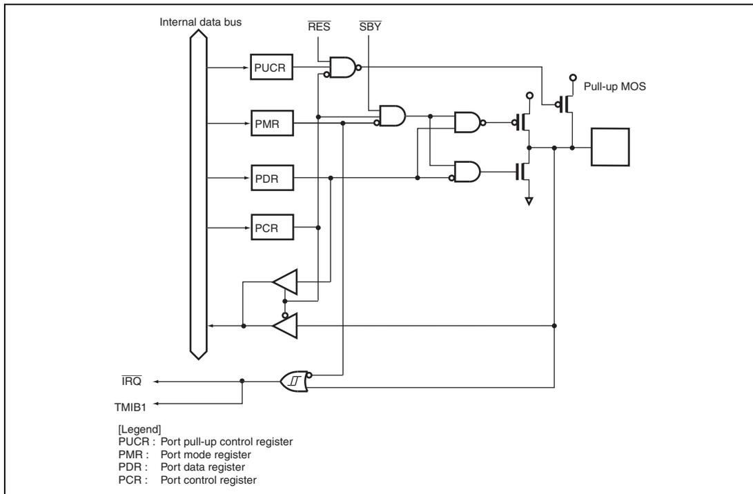
**Figure B.3 Port 1 Block Diagram (P15)**
