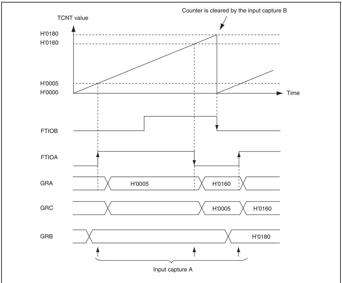
**Figure 13.40 Example of Buffer Operation (2)
