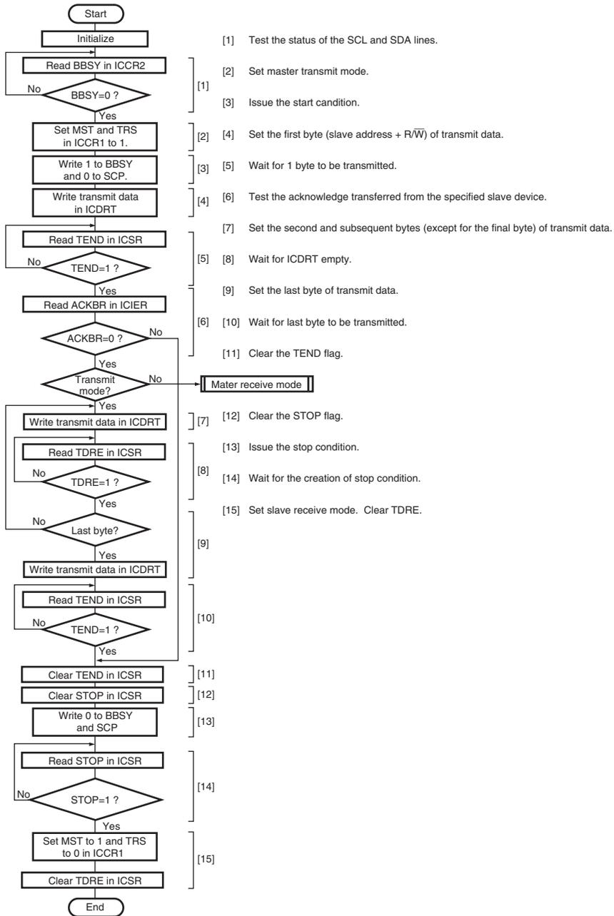
**Figure 17.17 Sample Flowchart for Master Transmit Mode**
