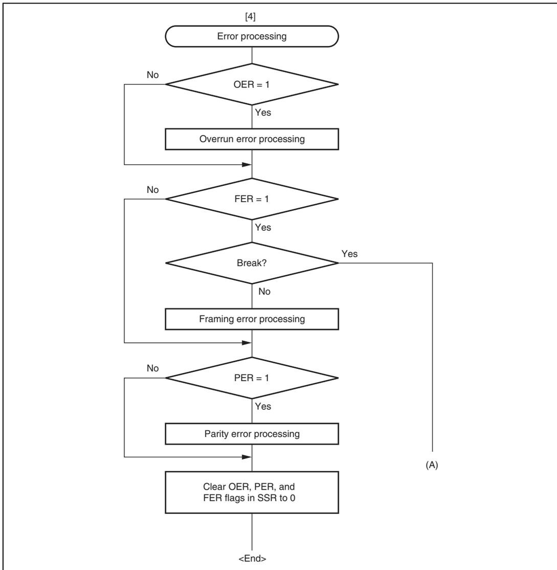
**Figure 16.8 Sample Serial Reception Data Flowchart (Asynchronous Mode) (2)**
