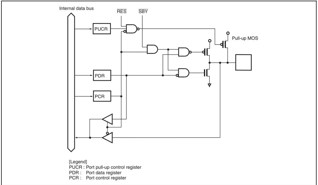
**Figure B.4 Port 1 Block Diagram (P12)**
