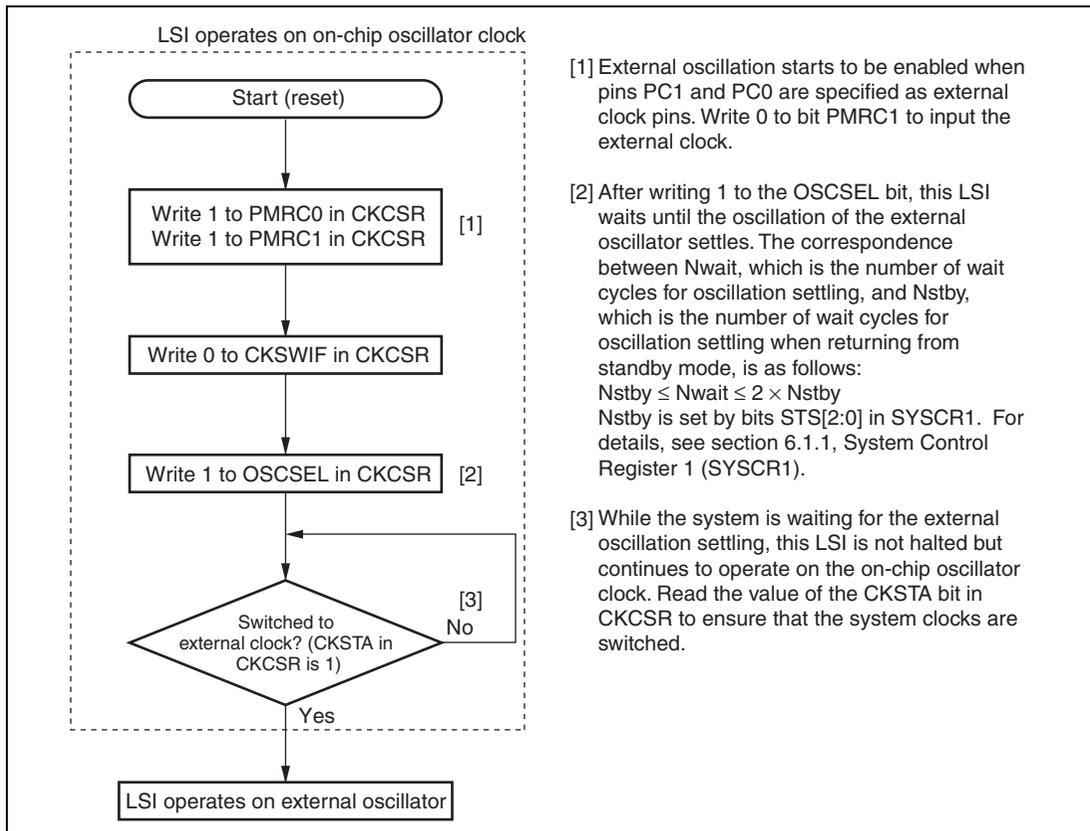
**Figure 5.4 Flowchart of Clock Switching with Backup Function Disabled (1)
