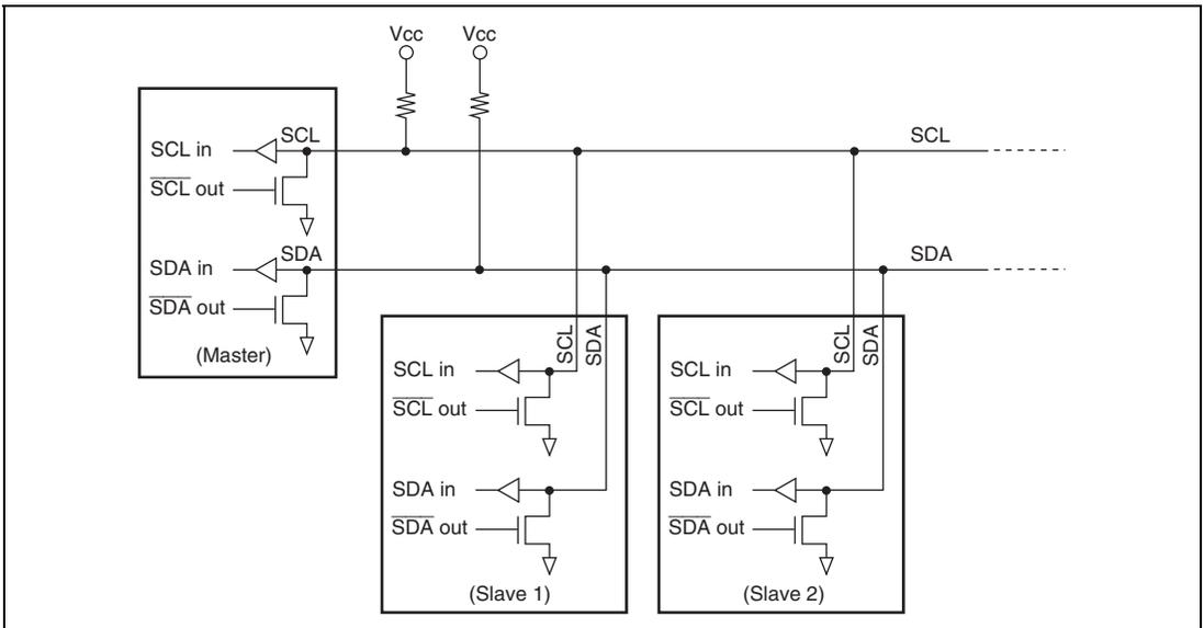
**Figure 17.2 External Circuit Connections of I/O Pins**
