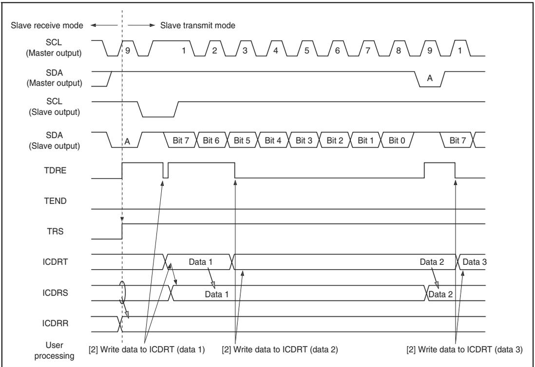
**Figure 17.9 Slave Transmit Mode Operation Timing (1)**
