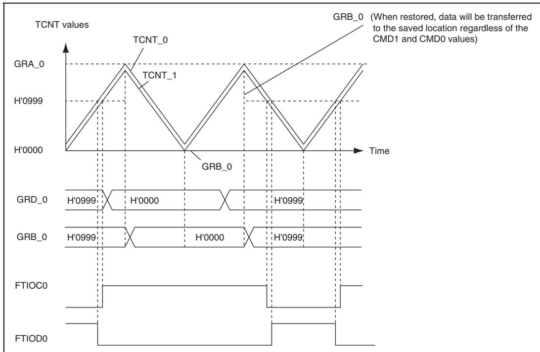
**Figure 13.43 Buffer Operation (4)**
