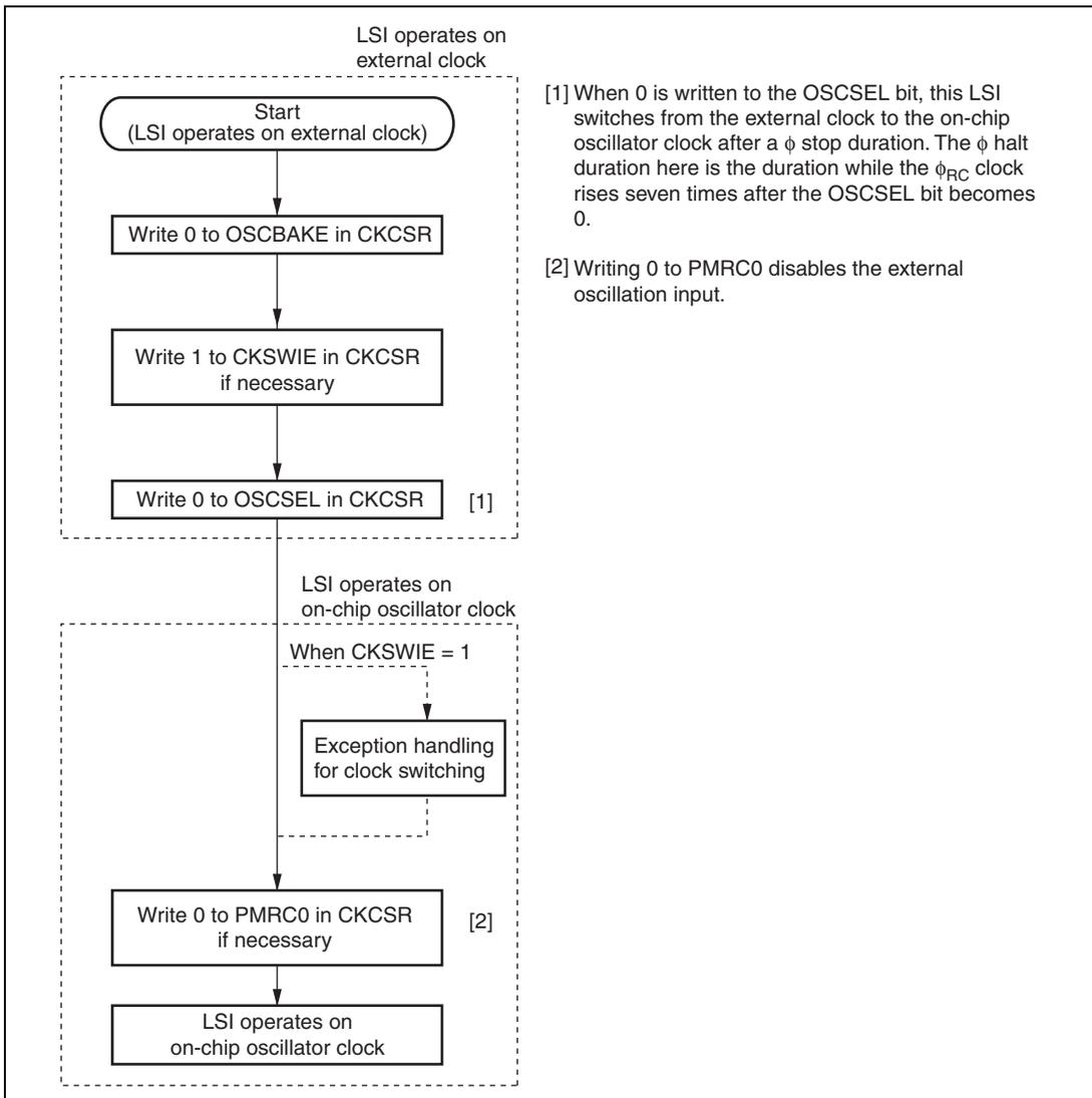
**Figure 5.5 Flowchart of Clock Switching with Backup Function Disabled (2)
