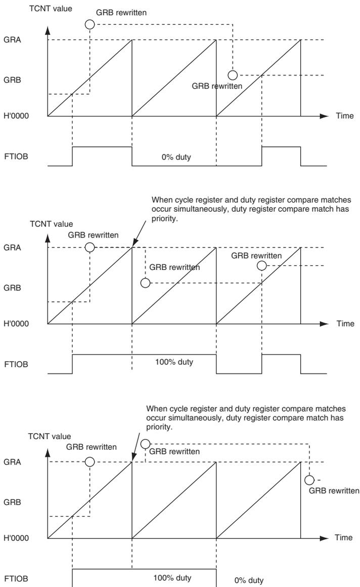
**Figure 13.25 Example of PWM Mode Operation (4)**
