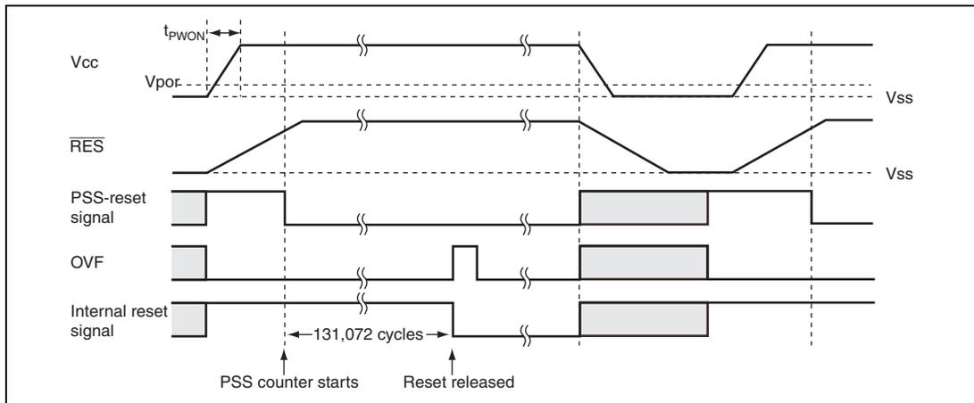
**Figure 19.3 Operational Timing of Power-On Reset Circuit**
