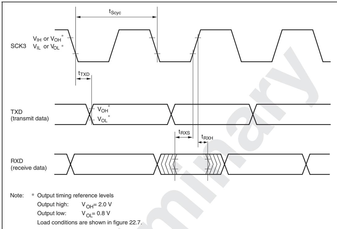
**Figure 22.6 SCI Input/Output Timing in Clocked Synchronous Mode**
