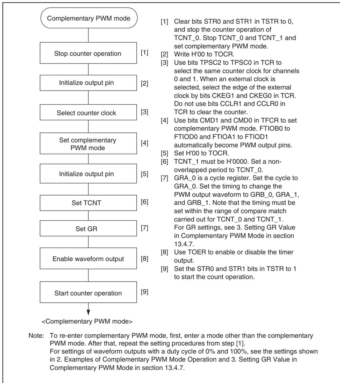
**Figure 13.29 Example of Complementary PWM Mode Setting Procedure**
