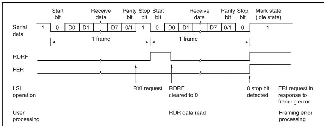
**Figure 16.7 Example of SCI3 Reception in Asynchronous Mode
