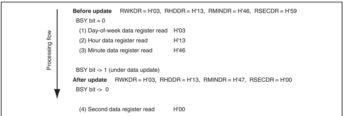
**Figure 10.4 Example: Reading of Inaccurate Time Data**
