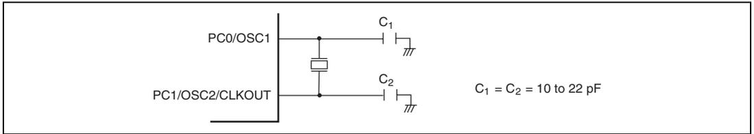
**Figure 5.11 Example of Connection to Crystal Resonator**
