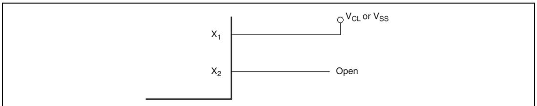
**Figure 5.18 Pin Connection when not Using Subclock**
