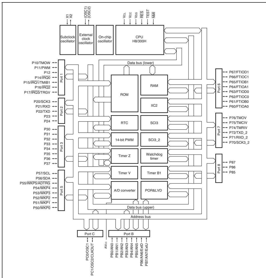
Figure 1.1 Block Diagram of H8/36077 Group
