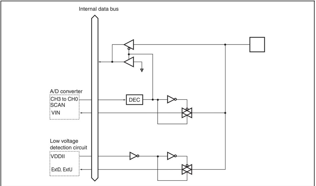
**Figure B.23 Port B Block Diagram (PB7 and PB6)**
