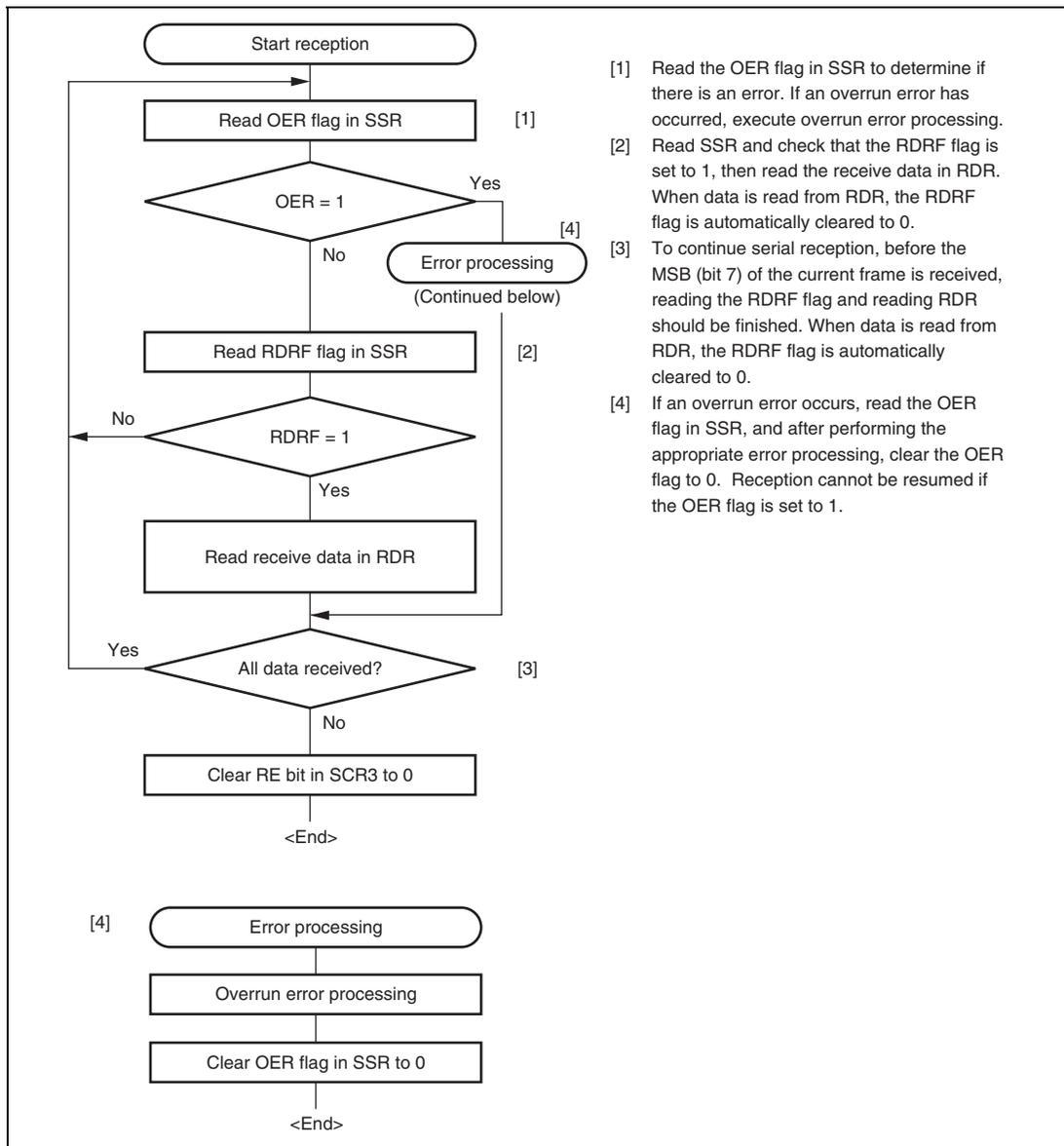
**Figure 16.13 Sample Serial Reception Flowchart (Clock Synchronous Mode)**
