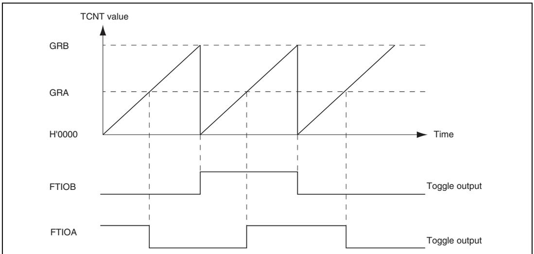
**Figure 13.14 Example of Toggle Output Operation**
