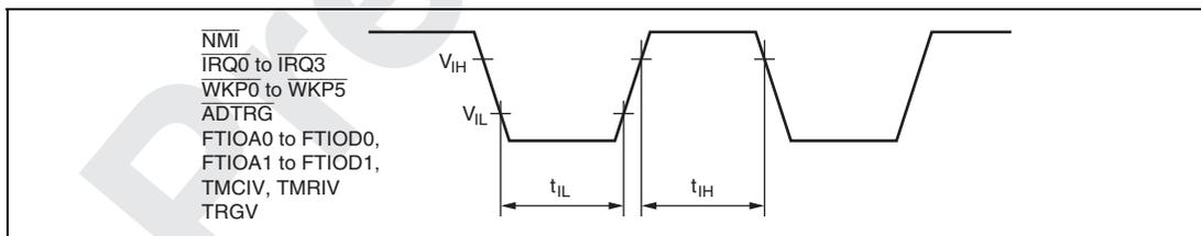
Figure 22.3 Input Timing
