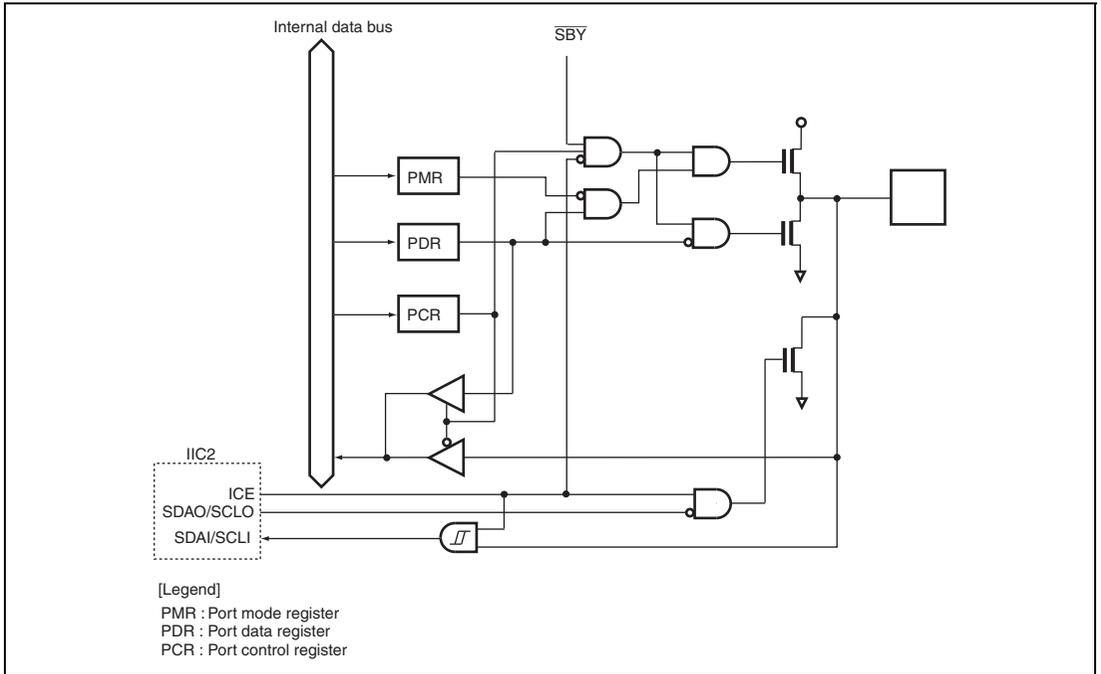
**Figure B.12 Port 5 Block Diagram (P57, P56)**
