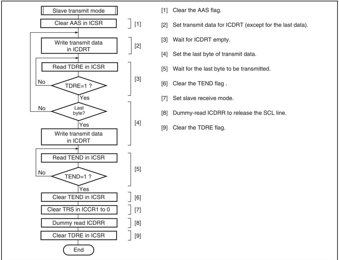
**Figure 17.19 Sample Flowchart for Slave Transmit Mode**
