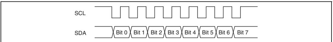
**Figure 17.13 Clock Synchronous Serial Transfer Format**
