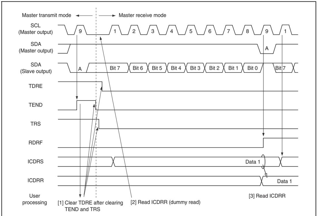
**Figure 17.7 Master Receive Mode Operation Timing (1)**
