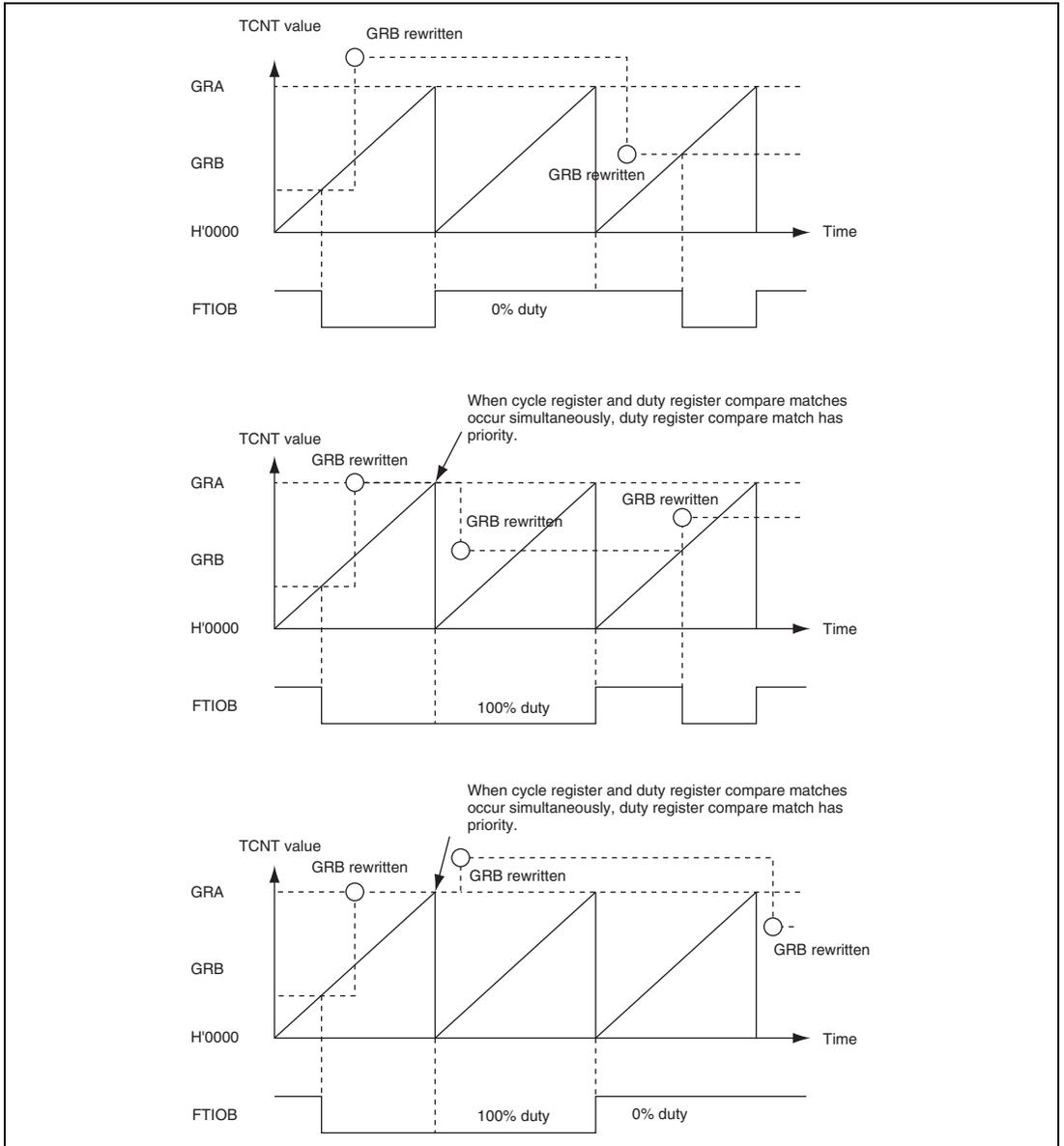
**Figure 13.24 Example of PWM Mode Operation (3)**
