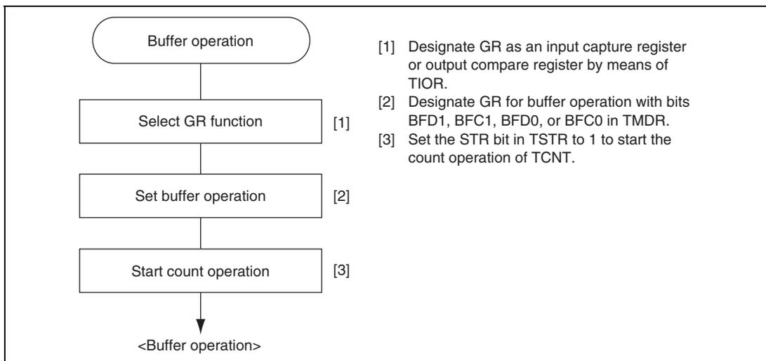
**Figure 13.37 Example of Buffer Operation Setting Procedure**
