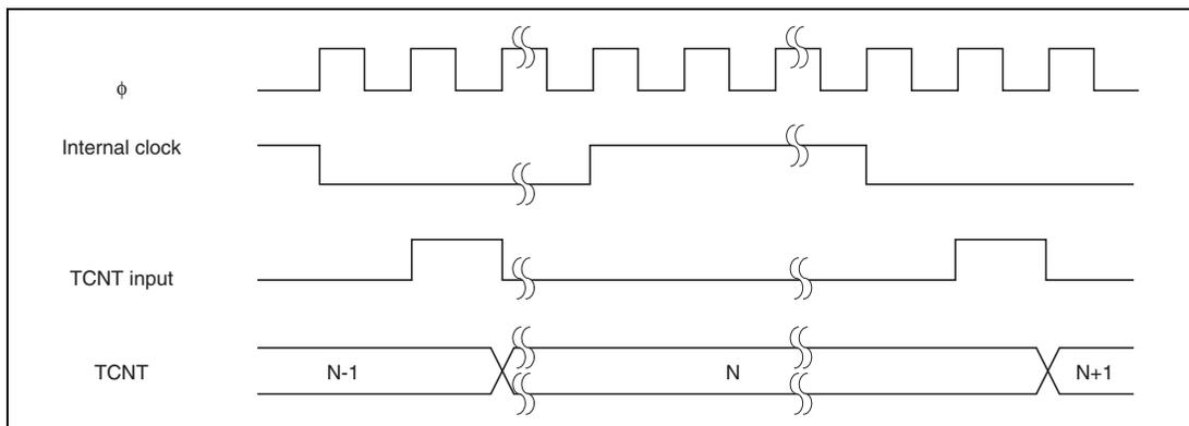
**Figure 13.10 Count Timing at Internal Clock Operation**
