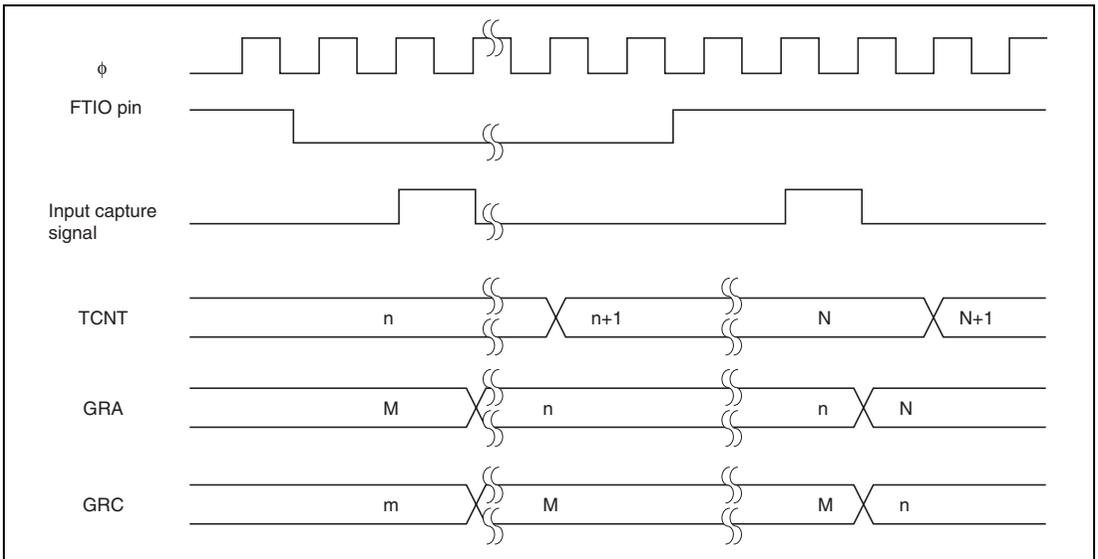
**Figure 13.41 Input Capture Timing of Buffer Operation**
