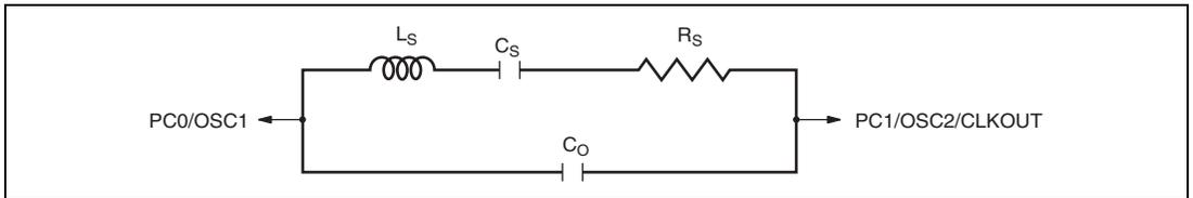
**Figure 5.12 Equivalent Circuit of Crystal Resonator**
