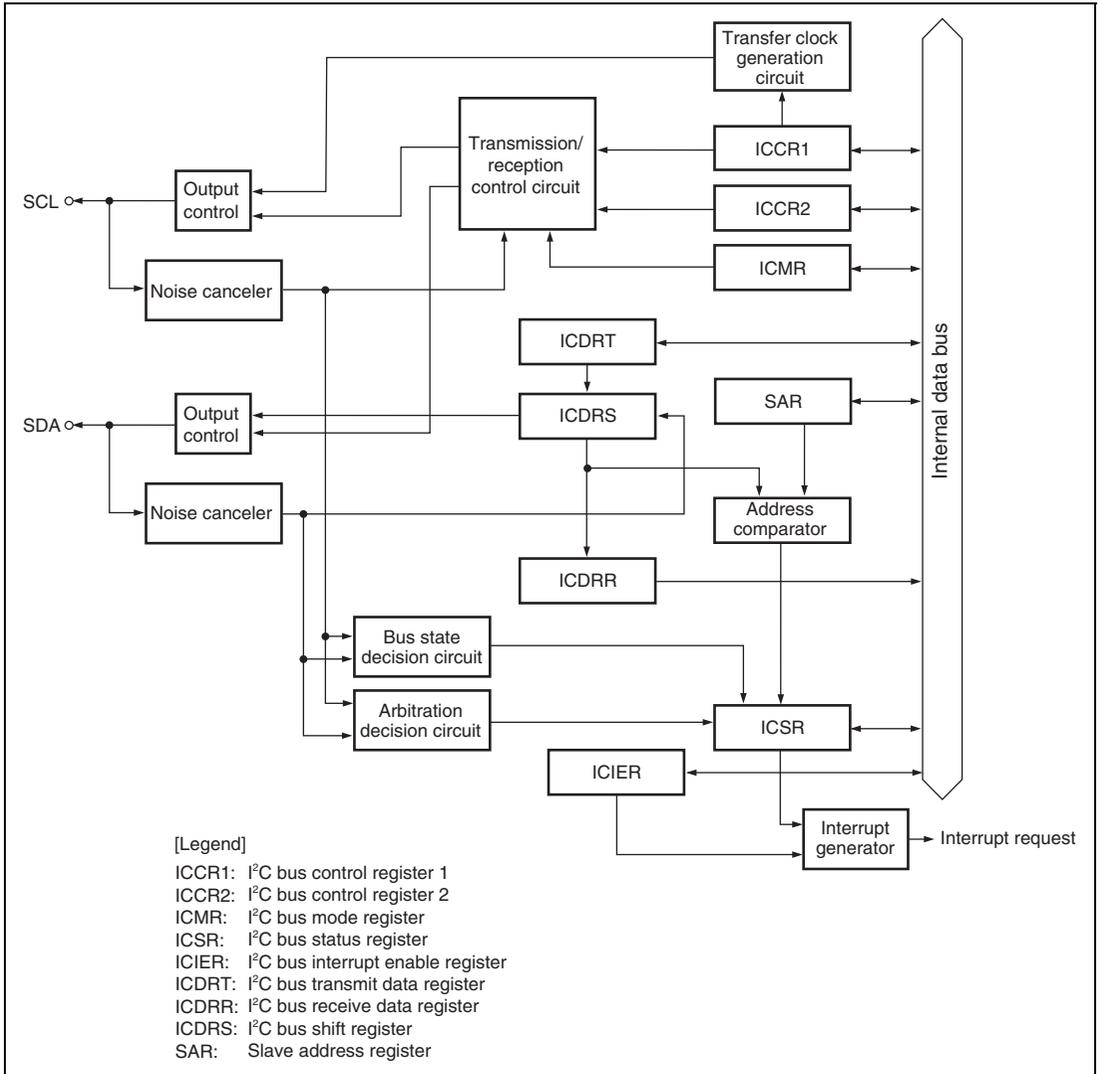
Figure 17.1 Block Diagram of I<sup>2</sup>C Bus Interface 2
