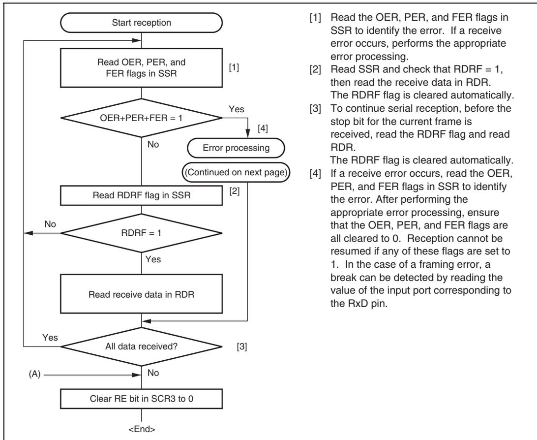
**Figure 16.8 Sample Serial Reception Data Flowchart (Asynchronous Mode) (1)**
