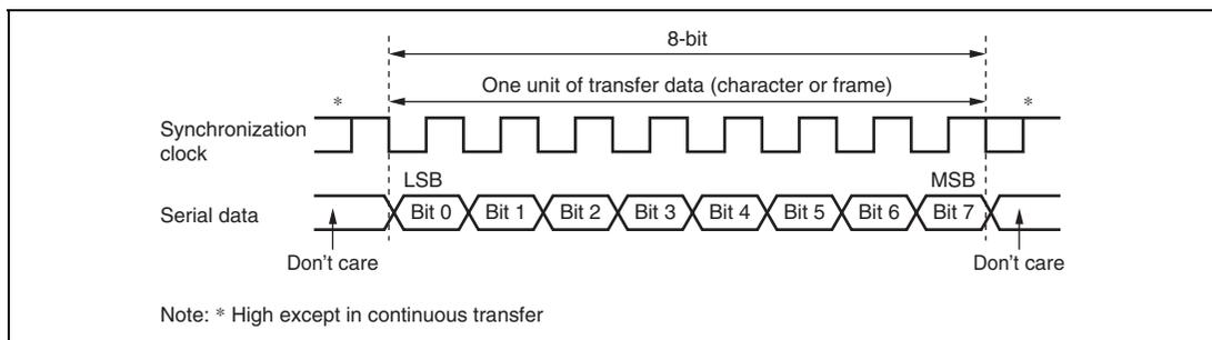
**Figure 16.9 Data Format in Clock Synchronous Communication**
