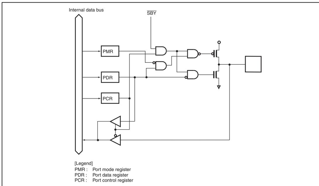
**Figure B.7 Port 2 Block Diagram (P24, P23)**
