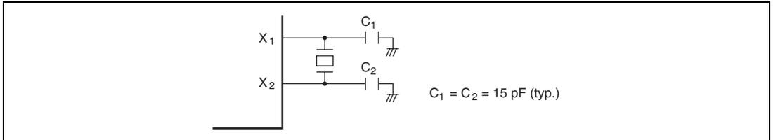
**Figure 5.16 Typical Connection to 32.768-kHz Crystal Resonator**
