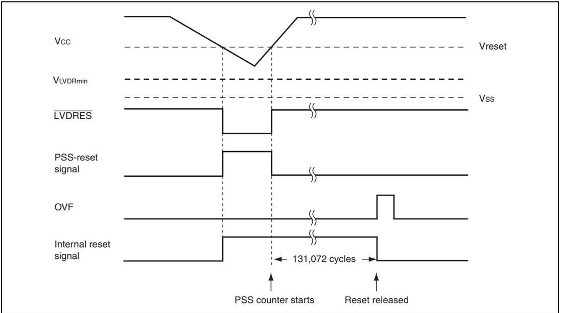
**Figure 19.4 Operating Timing of LVDR Circuit**
