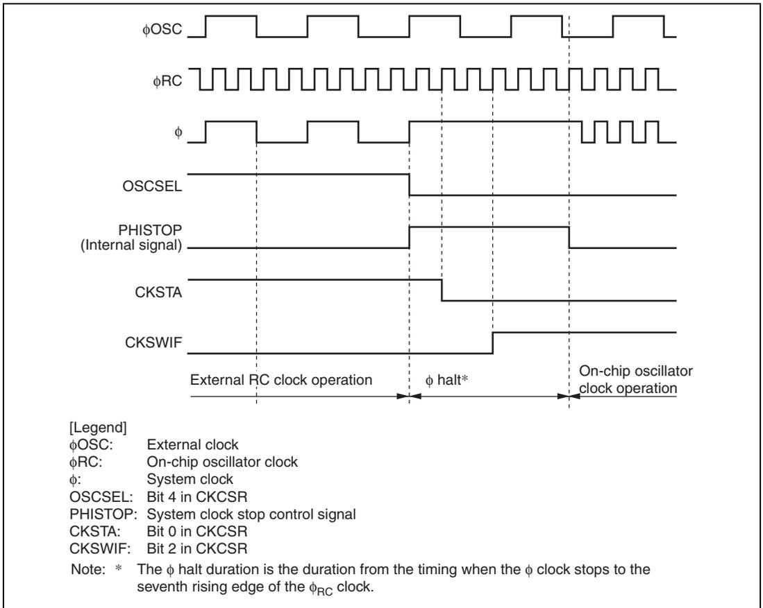
**Figure 5.7 Timing Chart to Switch from External Clock to On-Chip Oscillator Clock**
