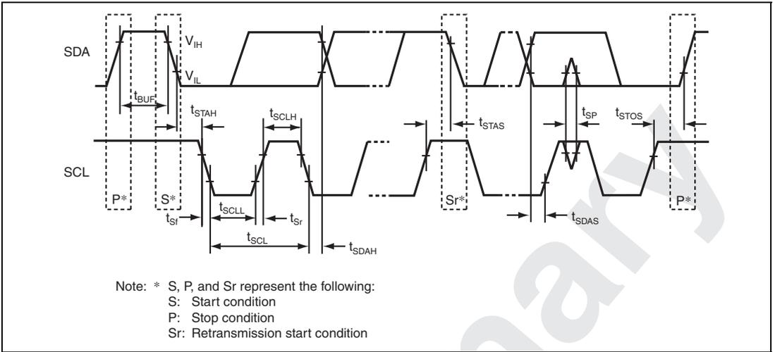
**Figure 22.4 I<sup>2</sup>C Bus Interface Input/Output Timing**
