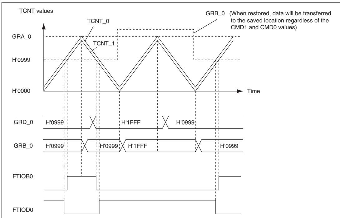
**Figure 13.42 Buffer Operation (3)**
