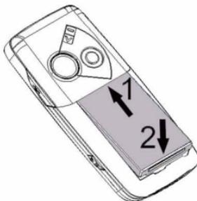
Close the case by locating the plastic cover horizontally into the grooves and *sliding* the cover up to close it. **DO NOT** force the cover down by pressing on it.
