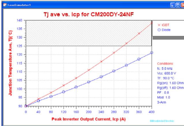
B) Power, Temperature vs. Current curve
