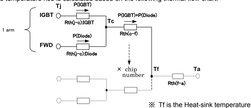
Temperature rise between junction (IGBT&FWD) and case is calculated to be
