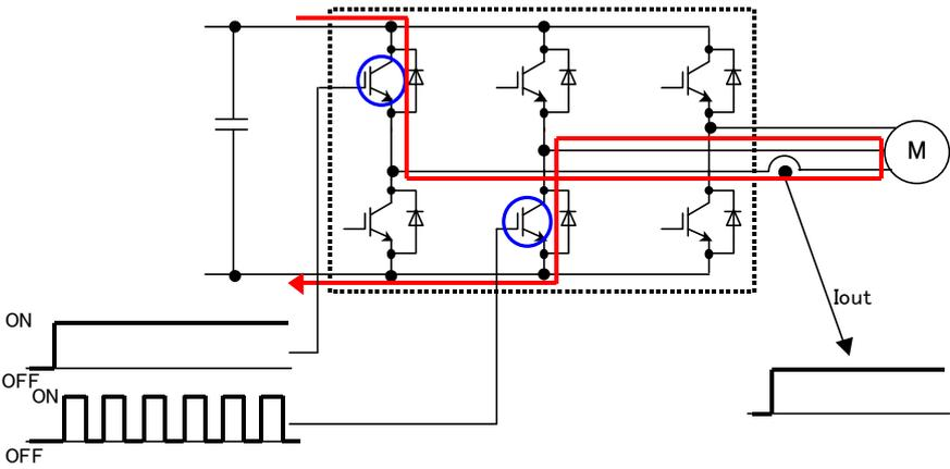
The power loss for chopper operation is calculated with the formulas shown below. No ripple component is included.
