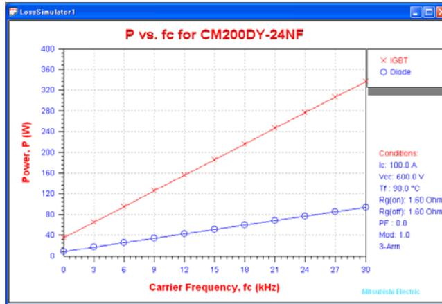
D) Power, Max. Current vs. Carrier Frequency curve
