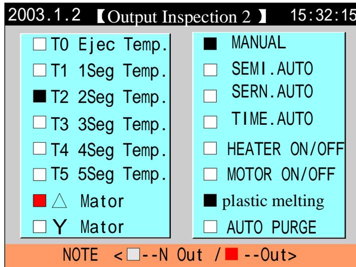
(4) Above delivery inspection pages are used for monitoring signals. If you want to inspect whether the delivery valve is ok or not manually without any actions, you can move the cursor to the delivery name which is waiting for your inspection, pressure 揺 nter 搦 utton, then the delivery valve will come to work. Meanwhile the solid block in the scene shows the delivery of the signals.
