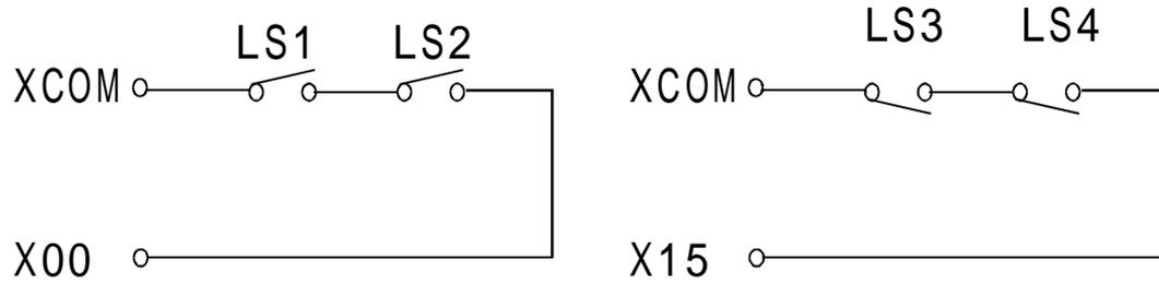
**Safety Door Wiring Diagram (for reference only)**
