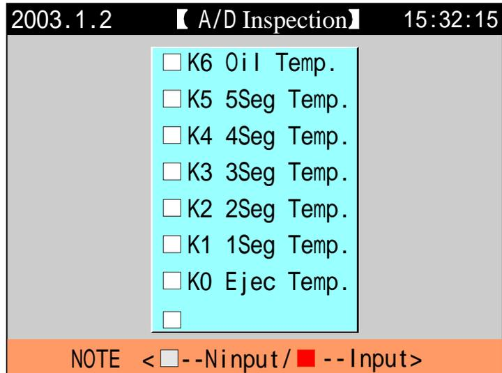
(6) The above input inspection pages are used for signal inspection and cannot accept information modification. The solid box on the display indicates that the signals are being input.
