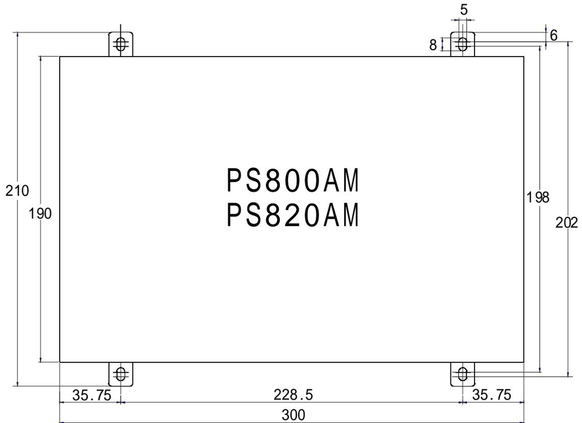
Exterior dimensions and installation hole position drawings for main controller
