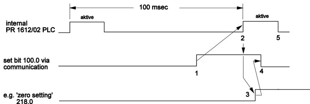
4. The internal PR 1612/02 PLC resets 100.0. This can be detected by the external PLC.
