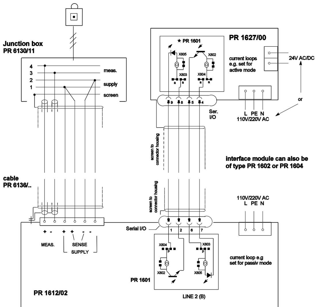
PR 1627/00 connectable to the PR1612/02 only via its line 2(B)
