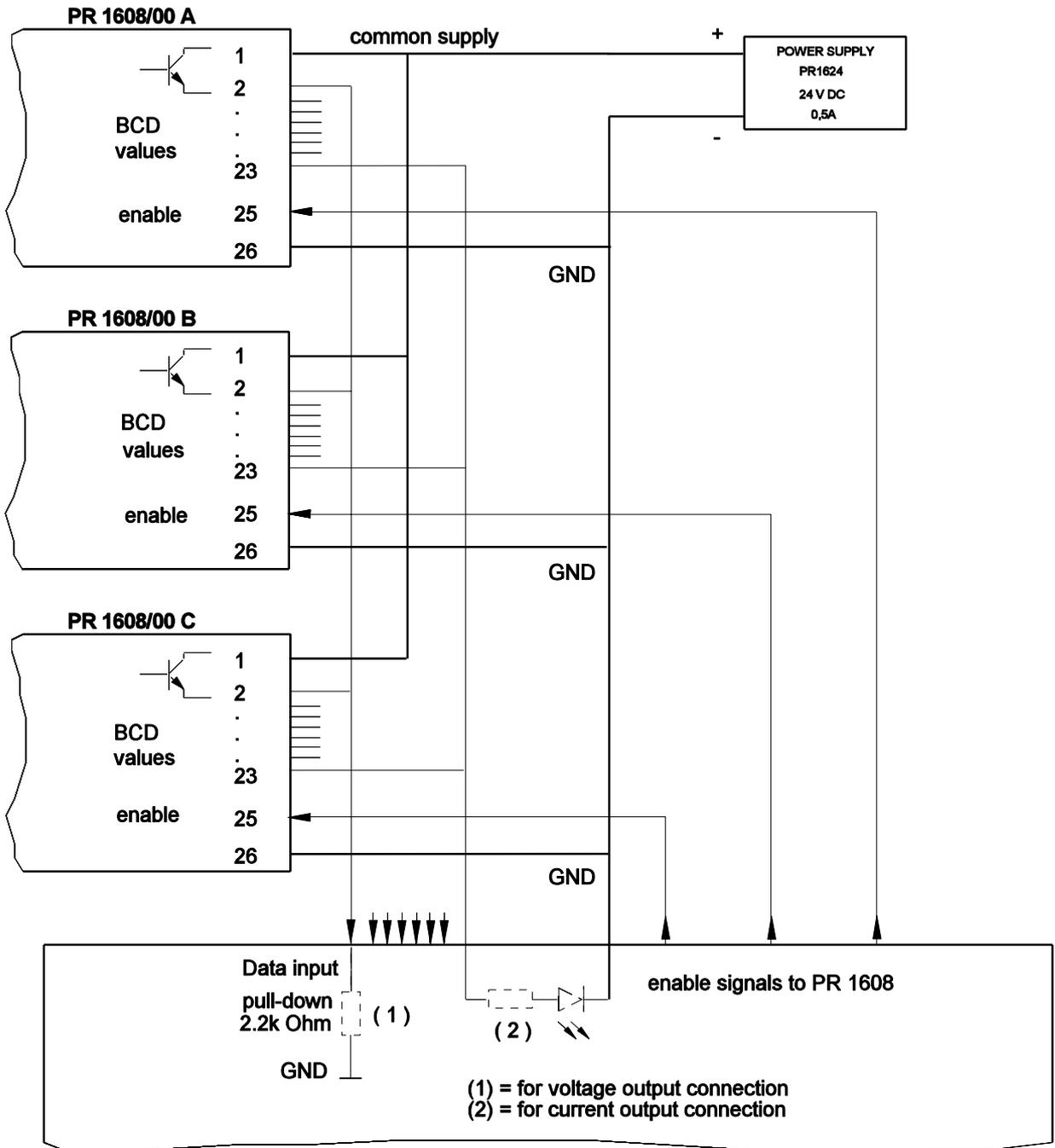
**7.11 OPTION PR 1608/10 (BCD/PLC output module with common ground)**
