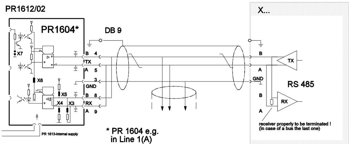
Settings at the PR 1604: solder links X3, X4, X5, X6 closed, solder link X7 open
