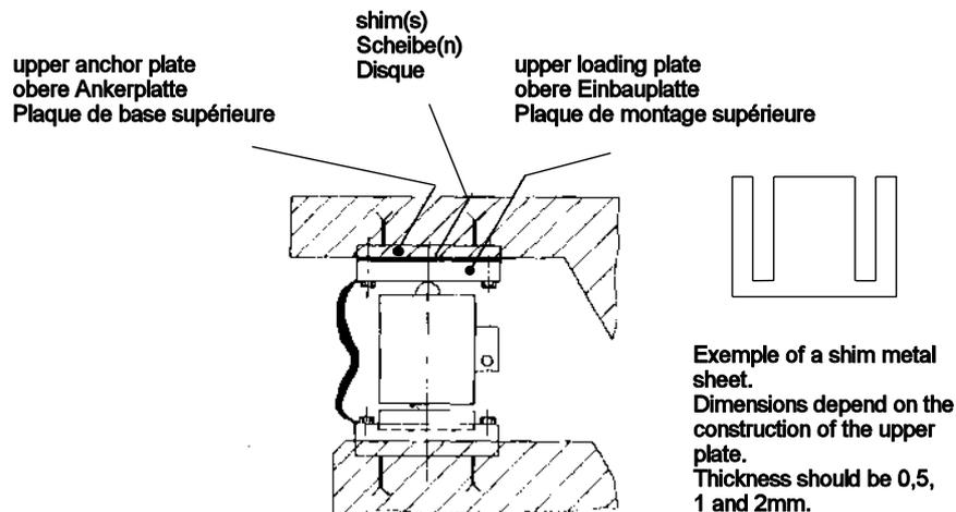
For shimming, lift up the platform close to the respective load cell and put a shim of 0.5 mm up to 2 mm thickness between upper loading and anchor-plate as drawn above.
