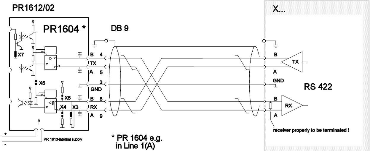
Settings at the PR 1604: solder links X3, X7 closed, solder links X4, X5, X6 open
