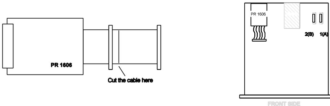
Before installing disconnect the mains voltage from the PR 1612/02 and cut the flat cable behind the first connector.
