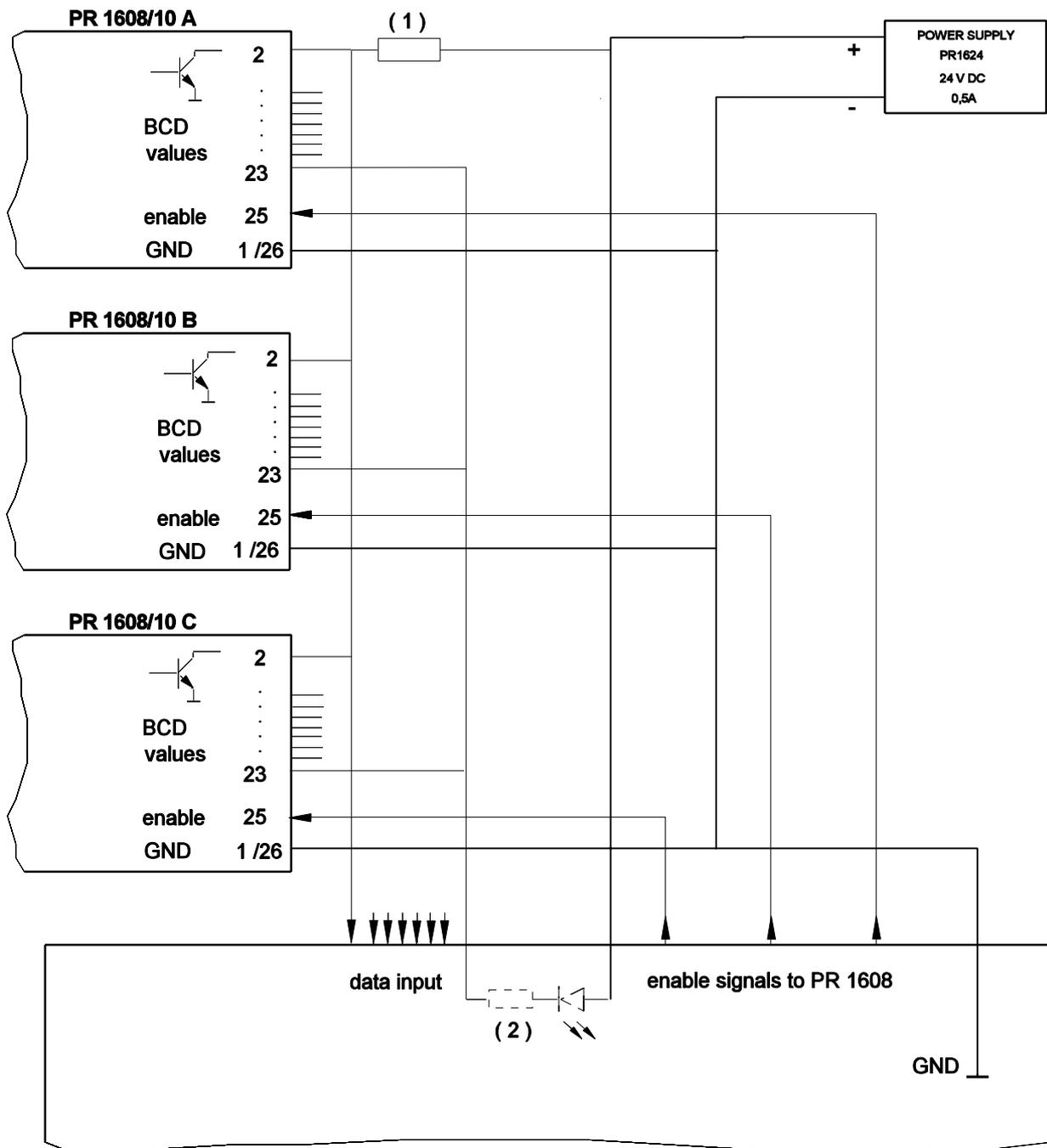
each output to be equipped with a pull-up resistor of
