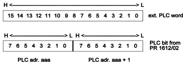
**Example:** Write command into the PR 1612/02 SPM, address 121 and value 8192
