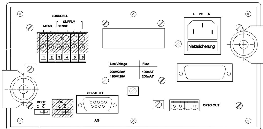
switch CAL must be sealed in position  $\bar{C}$
