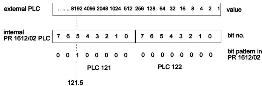
For setting bit 121.5 in PR 1612/02, value 8192 ( bit 5 in the upper byte of the word is set) must be written into the SPM.
