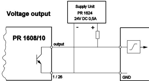
each output to be equipped with a pull-up resistor of
