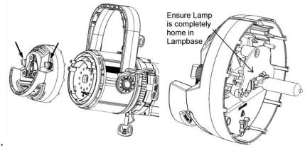
Isolate electrically before re-lamping the luminaire. Also be aware that the lamp and/or luminaire may still be hot, so exercise necessary caution to avoid burns.
