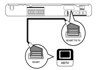
1 Connect a scart cable to the SCART TO TV jack on this Home Theater System and the SCART input jack on the TV.
