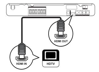
1 Connect an HDMI cable (not supplied) to the HDMI OUT jack on this Home Theater System and the HDMI input jack on the TV.
