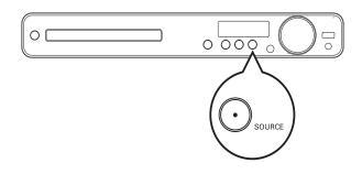
Press the SOURCE button repeatedly to select: DISC > USB > FM > SCART IN > AUX > COAX IN > OPTI IN > MP3 LINK > DISC ...
