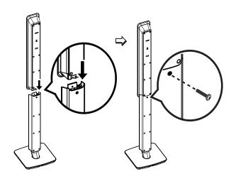
1 Attach the speakers to the speaker stands and secure the position with screws.
