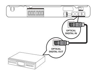
1 Connect an optical cable (not supplied) to the **OPTICAL DIGITAL-IN** jack on the Home Theater System and the OPTICAL/SPDIF output jack on the device.
