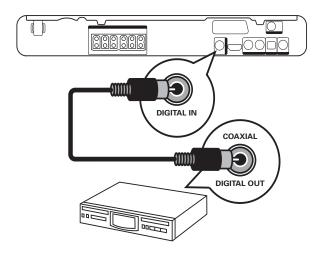
1 Connect a coaxial cable (not supplied) to the COAXIAL DIGITAL-IN jack on the Home Theater System and the COAXIAL/DIGITAL output jack on the device.
