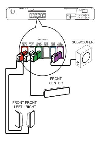
For HTS3270 and HTS3377 (HTS3270 has a different set of speakers)
