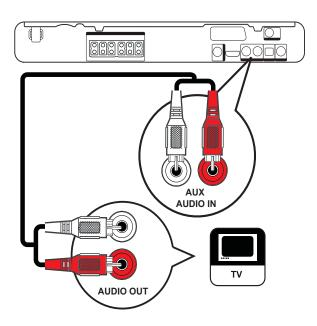
1 Connect the audio cables (not supplied) to the AUDIO IN-AUX jacks on the Home Theater System and the AUDIO output jacks on the TV.
