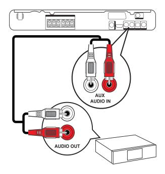
1 Connect the audio cables (not supplied) to the AUDIO IN-AUX jacks on the Home Theater System and the AUDIO output jacks on the device.
