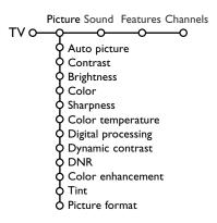
Note: Sharpness, Digital natural motion, Dynamic Contrast, DNR, Color enhancement, Tint and Picture format are not available for HD sources.
