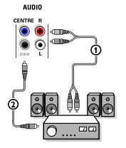
Connect the audio cable to the multi channel Surround receiver and to AUDIO RECEIVER L and R next to the CENTRE connector of your TV (1).
