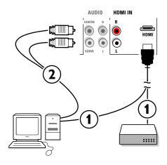
HDMI is the leading new standard for Digital High Definition video and audio interconnection. Eg. with a Digital Set top box, with HDMI-equipped devices like a PC, DVD-R, AV receiver...
