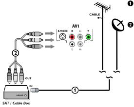
Connect the satellite antenna cable or the Cable TV cable (1) to the satellite receiver's or cable box's IN jack.
