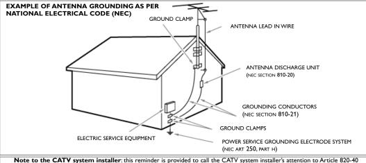
Note to the CATV system installer: this reminder is provided to call the CATV system installer's attention to Article 820-40 of the NEC that provides guidelines for proper grounding and, in particular, specifies that the cable ground shall be connected to the grounding system of the building, as close to the point of cable entry as practical.
