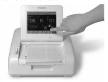
The monitor is operated using the touchscreen. All user functions (apart from the On/Off switch) are controlled directly from the screen, and the intuitive, color, graphical user interface not only makes it quick and easy to learn and use, but the lack of mechanical controls also makes cleaning the Avalon fetal monitor much quicker and simpler.
