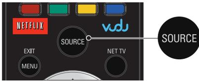
Press **SOURCE** repeatedly to select the set-top box or the connected device and wait a few seconds till the picture appears. (e.g.)
