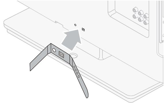
2 Pass cables through the cable management tie to avoid tangles.
