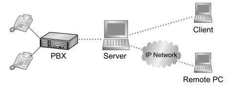
If Maintenance Console is installed on the client PC, a web server is not necessary.
