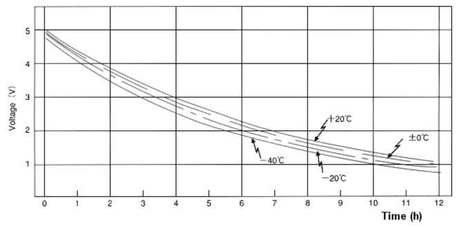
**Note:** At low temperatures, ion movement for the formation of electric double layers becomes slow and the time required to complete charging is longer. Consequently, in the case where there is no any difference in charging time, the lower the temperature the more the initial voltage drop.
