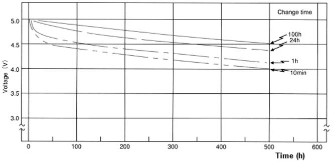
Note: If charging time is brief, complete charge is not attained, and initial voltage due to internal charge is increased.
