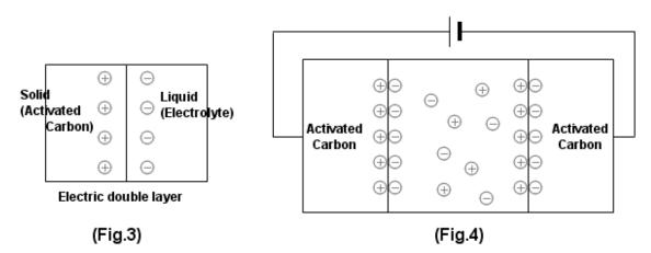
The electric double layer acts as an insulator and does not allow current to flow when an external DC voltage is applied. As the voltage level is increased, a point is reached where the current will begin to flow. The magnitude of this voltage is called the "decomposition voltage". Further increasing this voltage will cause the electrolyte to decompose causing additional current to flow.
