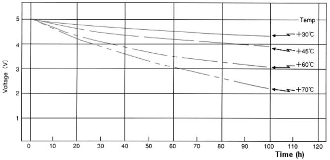
**Note:** At self-discharge, the terminal voltage drop is affected by ambient temperature. This means the self-discharge current increases as ambient temperature rises. In cases where it is used with a micro applied current of nano-ampere order, ambient temperature allows a difference to occur in back-up time.
