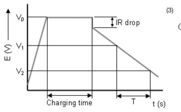
$C = \frac{I \times T}{(V_1 - V_2)}$  (Farad)
