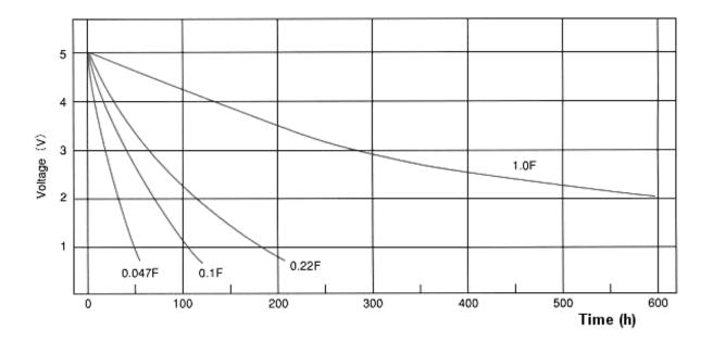
Constant resistance discharge Charge voltage: 5V Charge time: 24hours Part number: EECSoHD473V (5.5V0.047F)
