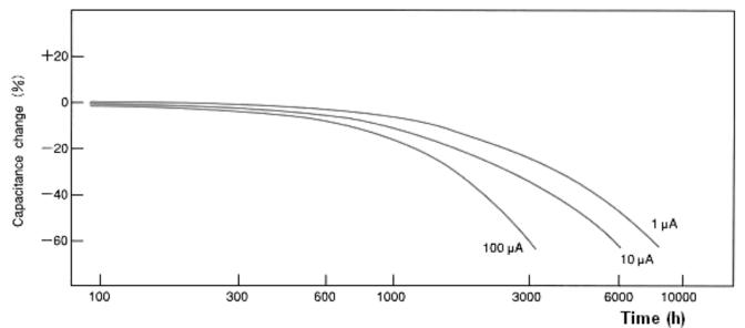
**Note:** Capacitance changes at life test vary based on applied current (measuring current). The longer the life, the less the applied current.
