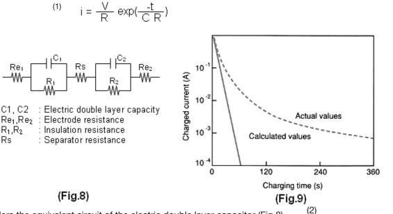
If one considers the equivalent circuit of the electric double layer capacitor (Fig.8) as having many small capacitors ( $C_n$ ) with various internal resistance ( $R_n$ ), then the current that flows through an individual capacitor can be represented by Equation 2.
