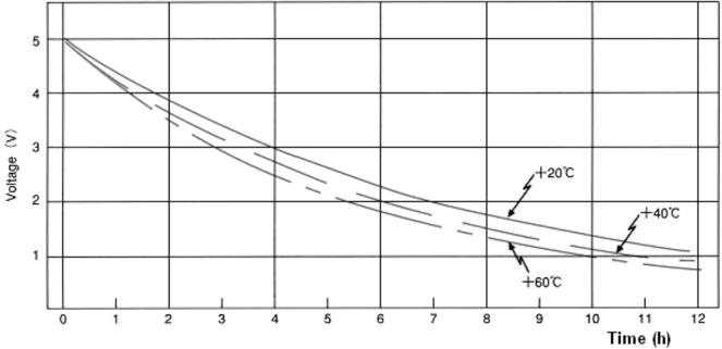
**Note:** Voltage drops faster as ambient temperature rises. This occurs because the rise in ambient temperature causes a self-discharge current to be added to the applied current.
