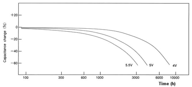
**Note:** Capacitance changes at the life test vary from applied voltage. The lower the voltage, the smaller capacitance becomes. There is almost no capacitance change due to no-load shelving.
