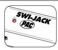
Once programming is completed, wait 7 seconds. The LED will flash three times indicating end of programming. The Interface will then flash the version number it was programmed for.
