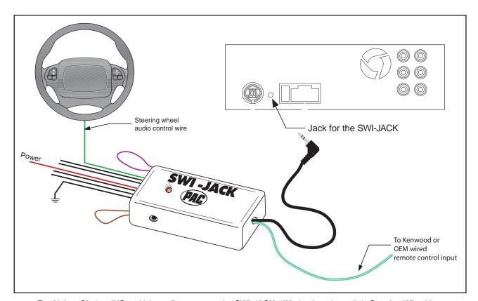
For Alpine, Clarion JVC, or Valor radios, connect the SWI-JACK 1/8" plug into the radio's Steering Wheel input jack on back of radio or wire harness. For Kenwood, or OEM radios, connect the blue/yel wire to the Remote Input wire (blue/yel for Kenwood, gray for OEM) of radio.
