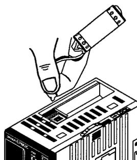
5. To enable the detection of low battery errors, slide the Low Battery Detection Switch towards the front of the Unit and set bits 12 to 15 of DM 6655 to "0."
