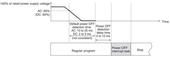
**Note** The execution time of the program in the power OFF interrupt task must be less than 10 ms minus the power OFF detection delay time. For information on power OFF interrupt tasks, refer to 5-2-3 Interrupt Tasks. For information on operation at power OFF, refer to A-5 Operation for Power Interruptions.
