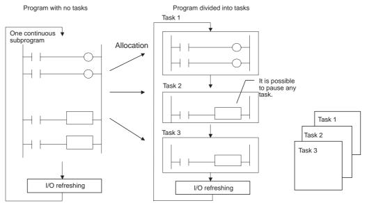
A program without tasks is like reading an entire scroll form the beginning, while a program with tasks is like reading cards individually. Each card can enable or disable other cards. Reading disabled cards will be skipped.
