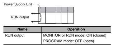
This RUN output can be used to create an external safety circuits, such as an emergency stop circuit that prevents an Output Unit's external power supply from providing power unless the PLC is ON.
