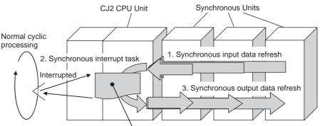
Write a program for synchronous unit operation, such as for digital cam control.
