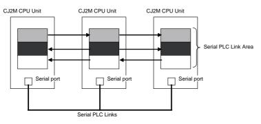
Words in the Serial PLC Link Area that are not allocated to Serial PLC Links can be used only in the program as work bits. Bits in the Serial PLC Link Area can be force-set and force-reset.
