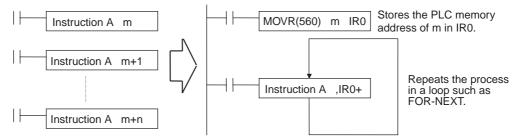
The following example shows how an Index Register in a program loop can replace a long series of instructions. In this case, instruction A is repeated n+1 times to perform some operation such as reading and comparing a table of values.
