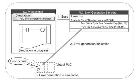
**Note** Unlike with an actual error, ladder execution will not stop even if a fatal error is generated using the PLC error generation simulation function.
