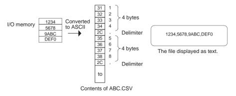
Structure of CSV and TXT Data Files with Double-word Fields
