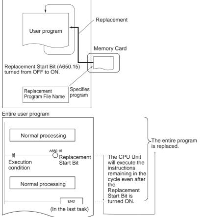
The program can also be replaced when program execution is stopped (PROGRAM mode) by turning ON the Replacement Start Bit from the CX-Programmer.
