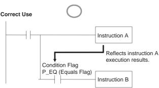
The same execution condition (a) is used for instructions A and B to execute instruction B based on the execution results of instruction A. In this case, instruction B will be executed according to the Condition Flag only if instruction A is executed.
