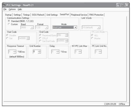
The following parameters are valid when pin 5 on the DIP switch on the CPU Unit is OFF (default).
