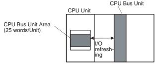
Each CPU Bus Unit is allocated 25 words based on its unit number, as shown in the following table.
