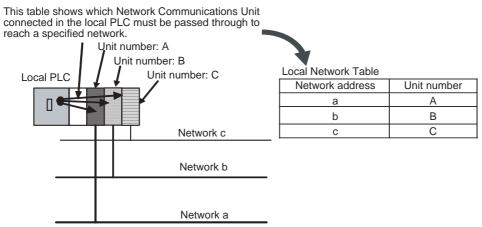
The local network table gives the unit number of the Network Communications Unit connected in the local PLC and the corresponding address of the FINS network connected to that Unit for FINS communications.
