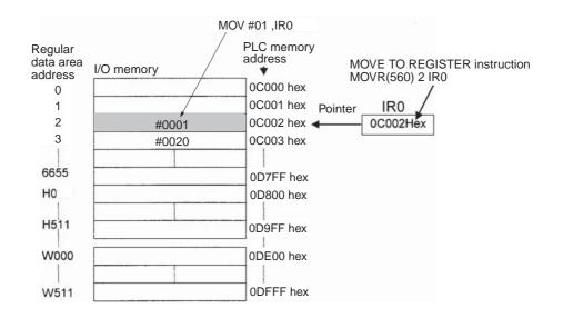
**Note** The PLC memory addresses are listed in the diagram above, but it isn't necessary to know the PLC memory addresses when using Index Registers.
