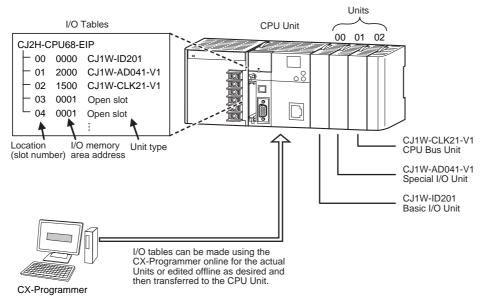
The CPU Unit automatically verifies with the connected Units (actual I/O tables) mounted to it according to this data.
