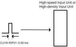
Inputs that are input to internal memory are cleared when the inputs are refreshed.
