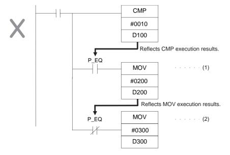
The Equals Flag will turn ON if D100 in the rung above contains #0010. #0200 will be moved to D200 for instruction (1), but then the Equals Flag will be turned OFF because the #0200 source data is not 0000 Hex. The MOV instruction at (2) will then be executed and #0300 will be moved to D300. A rung will therefore have to be inserted as shown below to prevent execution results for the first MOV instruction from being picked up.
