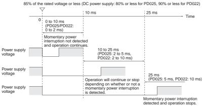
Note The above timing chart shows an example when the power OFF detection delay time is set to 0 ms.
