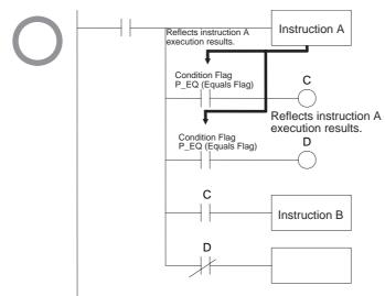
**Example:** The following example will move #0200 to D200 if D100 contains #0010 and move #0300 to D300 if D100 does not contain #0010.
