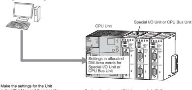
Make the settings for the Unit in the I/O tables and then transfer the settings to the CPU Unit.
