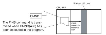
Note FINS commands can be transmitted to Special I/O Units in other PLCs in the network, not just the local PLC.
