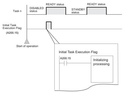
The Initial Task Execution Flag will turn ON when a task is executed the first time. Use this flag to trigger initializing processing.
