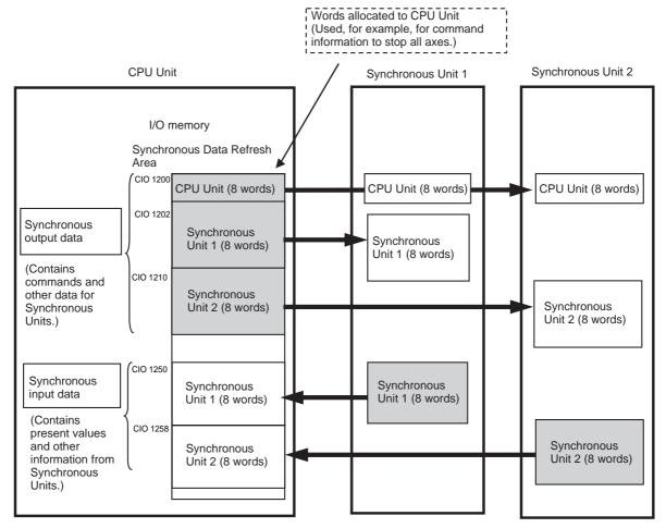
The following settings are made in the *Synchronous Unit Operation Settings* Area of the Timings/Synchronous Tab Page in the PLC Setup.
