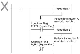
Make sure each of the results is picked up once by an OUTPUT instruction to ensure that execution results for instruction B will be not be picked up.
