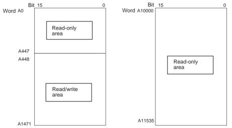
The following operations can be performed from the CX-Programmer to write data in the Auxiliary Area: Changing present values when monitoring programming addresses (set values dialog box), or transferring data to the PLC after editing the PLC data tables. Also the online set/reset operation cannot be used for bits in the Auxiliary Area. Refer to the *CX-Programmer Operation Manual* (Cat. No. W414).
