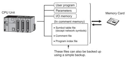
This enables backup/restoration of all data in the CPU Unit including I/O comments if an error occurs or when adding a CPU Unit with the same specifications without requiring the CX-Programmer.
