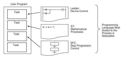
You can use the best language for each process by using different languages for different purposes, such as ladder programming for the device control or ST for mathematical processing.
