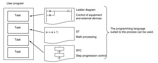
In addition, ladder diagrams and ST language can be freely used for function blocks (FBs) in ladder diagrams and ST programs, and for transition and action programs in SFC. This feature makes it possible to optimize structured programming.
