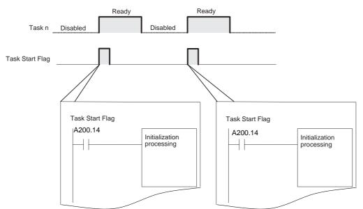
The Task Start Flag can be used to perform initialization processing whenever a task goes from STANDBY to READY status, i.e., when a task on STANDBY is enabled using the TKON(820) instruction.
