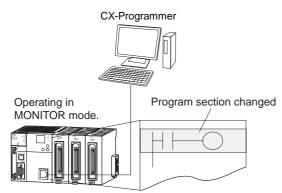
The cycle time will be increased by from one to several cycle times if the program in the CPU Unit is edited online in MONITOR mode.
