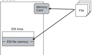
With the CJ-series PLCs, Memory Cards and a specified range of the EM Area can be used as memory to store files. Either can be used to save the entire user program, I/O memory, and parameter areas as files.
