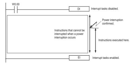
2 Set the Disable Setting for Power OFF Interrupts in A530 to A5A5 Hex to enable disabling power interruption processing.
