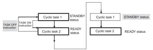
If a TASK OFF instruction is executed for its own task, the task will stop being executed where the TASK OFF instruction is executed, and the task will change to STANDBY status.
