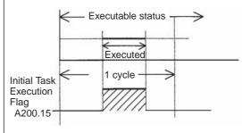
A200.15 will turn ON during the first time a task is executed after it has reached executable status. It will be ON only while the task is being executed and will not turn ON if following cycles.
