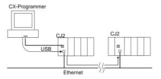
Connect online to a PLC on a network from a personal computer connected directly to the network.
