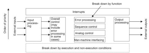
• Break down and design programs to ensure autonomy. Keep the amount of data exchanged between tasks to an absolute minimum.
