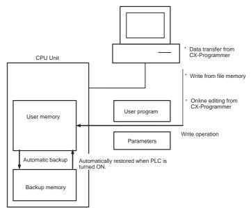
The BKUP indicator on the front of the CPU Unit will light while data is being written to backup memory. When transferring the user program from the CX-Programmer or transferring data to the parameter area from file memory, do not turn OFF the power to the CPU Unit until the backup operation has been completed (i.e., until the BKUP indicator turns OFF). The following table shows the operations that will be performed if the power is turned OFF before the backup is completed.
