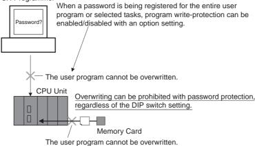
If the selected tasks or program are write-protected by selecting this option when registering a password, only the tasks (program) that are password-protected will be protected from overwriting. It will still be possible to overwrite other tasks or programs with operations such as online editing and task downloading.
