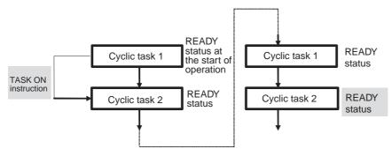
A cyclic task that is in STANDBY status will maintain that status in subsequent cycles. The task will have to be turned ON using a TASK ON instruction in order to switch from STANDBY status to READY status.
