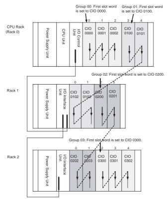
For example, a first slot word has been set in the middle of each Rack. Only 16-point Units have been used.
