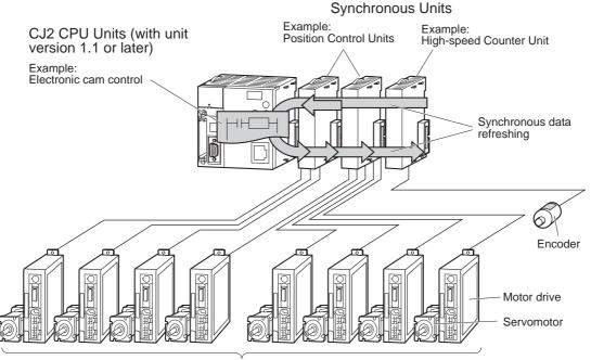
Several servomotors are controlled synchronously based on the operation of the encoder.
