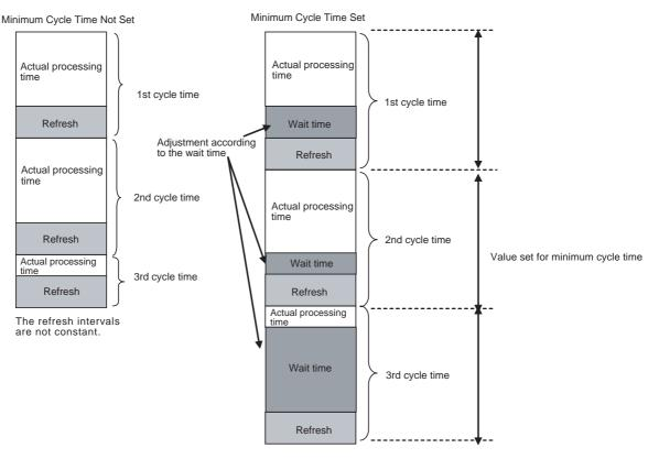
The I/O will be refreshed within the time set for the minimum cycle time.
