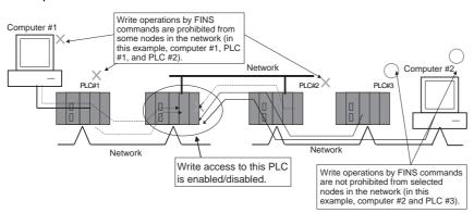
**Note** This function prohibits writing by FINS commands only, so it has no effect on write operations by functions other than FINS commands, such as data links.
