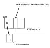
\*A "FINS Network Communications Unit" indicates a Controller Link Unit, SYSMAC LINK Unit, Ethernet Unit, DeviceNet Unit, or FL-net Unit. CompoNet Units are not included. It also indicates using the Serial Gateway for serial communications together with routing tables.
