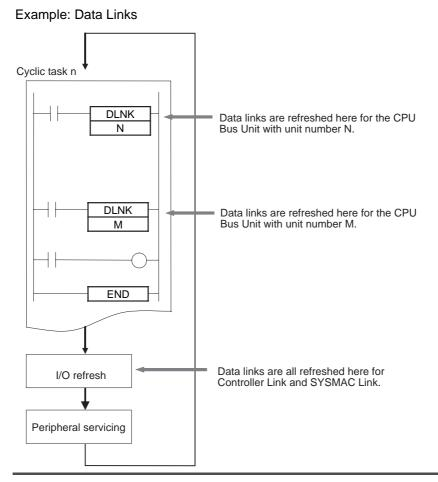
If DLNK(226) is executed for a CPU Bus Unit that is busy refreshing data, data will not be refreshed and the Equals Flag will turn OFF. Normally, the Equals Flag should be programmed as shown below to be sure that refreshing has been completed normally.
