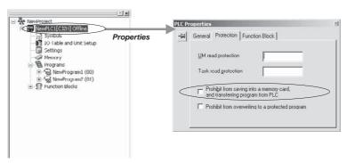
2 Either select *PLC - Transfer - To PLC* to transfer the program or select *PLC - Protection - Set Password* and click the OK Button.
