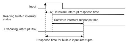
Response time for built-in input interrupts = Hardware interrupt response time + Software interrupt response time
