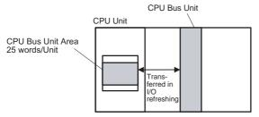
**Note** The CPU BUS I/O REFRESH instruction (DLNK(226)) can be executed in the ladder program to refresh the CIO Area words allocated to the CPU Bus Unit of a specified unit number.
