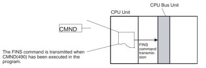
Note FINS commands can be transmitted to CPU Bus Units in other PLCs in the network, not just the local PLC.
