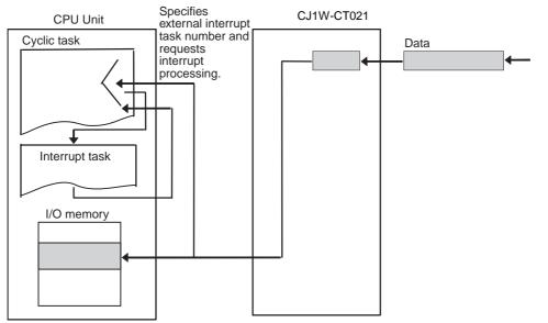
To communicate to the CPU Unit the status information for the two external control inputs and 32 outputs of this Unit for other than I/O refreshing, set the external control inputs or outputs so that they trigger the external interrupt task.
