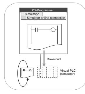
In addition to transferring programs and monitoring, the following functions can be used with the simulator. For details on the debugging procedure, refer to the *CX-Programmer Operation Manual* (Cat. No. W446).
