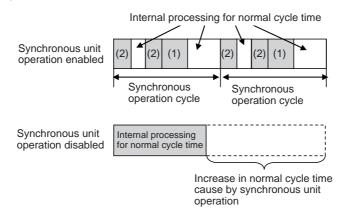
**Note** The above times are the same as the synchronous processing time minus the normal processing time performed during that time.
