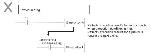
In this case then, instructions A and B are not differentiated instructions, the DIFU (of DIFD) instruction is used instead as shown below and instructions A and B are both upwardly (or downwardly) differentiated and executed for one cycle only.
