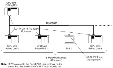
Note: If PTs are set to the Serial PLC Link protocol on the same line, the maximum of 8 Unit must include the polled PTs and CPU Units.
