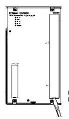
Use a standard screwdriver to remove the Memory Pack compartment cover.
