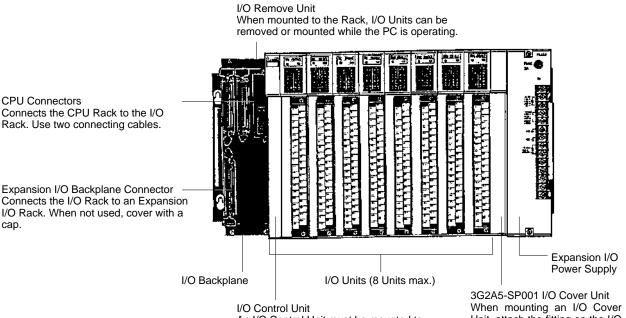
An I/O Control Unit must be mounted to the I/O Backplane in order to connect the I/O Backplane to Expansion I/O Racks. 3G2A5-SP001 I/O Cover Unit When mounting an I/O Cover Unit, attach the fitting on the I/O Backplane and the fitting on the back of the I/O Cover Unit.
