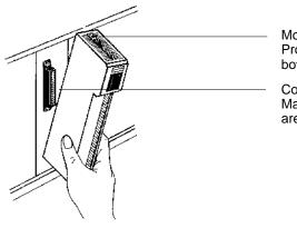
Mounting screws Provided at the top and bottom of the Unit
