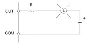
**Transistor Output Residual** When connecting TTL circuits to transistor Output Units, connect a pull-up resistor and a CMOS IC between the two. This is because of the residual voltage left on the transistor output after the output turns OFF.
