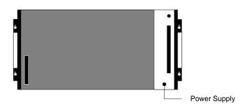
The core of the PC is the CPU. The CPU contains the program consisting of the series of steps necessary for the control task. The CPU fits into the position directly to the left of the Power Supply.
