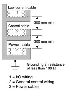
If the I/O wiring and power cables must be placed in the same duct (for example, where they are connected to the equipment), shield them from each other using grounded metal plates.
