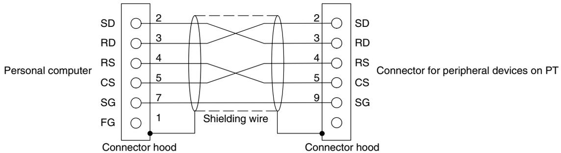
**Note** Please connect the shielding wire to the connector hood at both the personal computer and the peripheral device connector on the PT.
