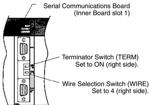
**Setting the Switches on an RS-422A Adapter**
