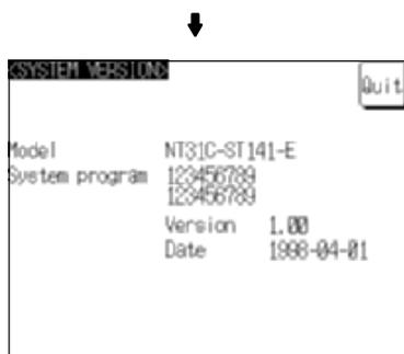
The system program's version information will be displayed as described below. Press the Quit touch switch to exit the Version Display screen and return to the Expansion Mode screen.
