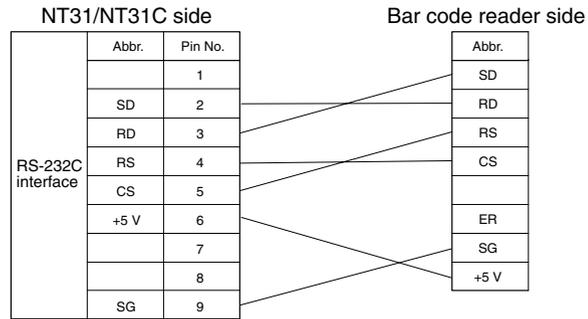
When using the +5 V output of the NT31/NT31C, limit the cable length to within 2 m. If a cable longer than 2 m is used, connect an external power supply to the bar code reader.
