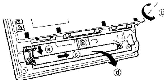
5. Fit a new CFL unit by following the procedure described below.
