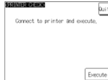
Confirm that a printer is connected to the NT31/NT31C, then press Execute: Printer Interface Check will be printed out at the printer.
