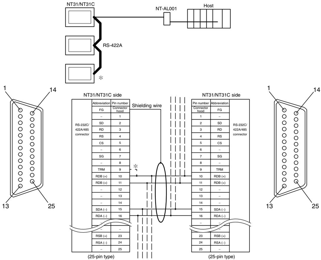
\*2 Make the connection between pin numbers 9 and 10 at the terminal NT31/NT31C (marked \* in the figure above) only.
