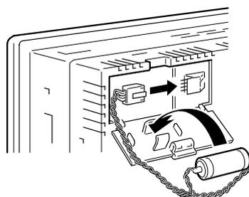
5. Close the battery cover, making sure that the cable is not trapped.
