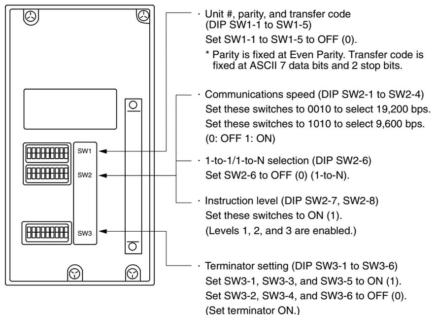
**Connecting to a CVM1/CV Series Host Link Unit****CVM1/CV series rack-mounting type: CV500-LK201**
