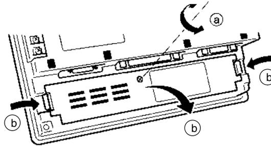
4. Remove the CFL unit by following the procedure described below.
