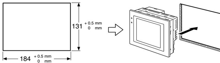
2. Attach the panel fittings at the four positions at top and bottom and two positions at right and left, shown below, from the rear of the NT31/NT31C.
