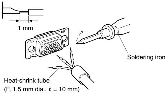
4. Push the heat shrink tube over the soldered joint and heat the tube to shrink it in place.
