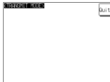
4. Open the screen data to be transmitted at the Support Tool, then select Download (NTST PT) in the Support Tool's Connect menu and specify the data to be transmitted.
