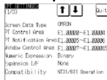
Switch the screen as required by pressing the [↓] (next screen) or [↑] (previous screen) touch switch.
