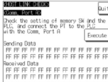
Press Execute to start the check. The data for checking communication is sent to the host, and is displayed as the Sending Data in hexadecimal.
