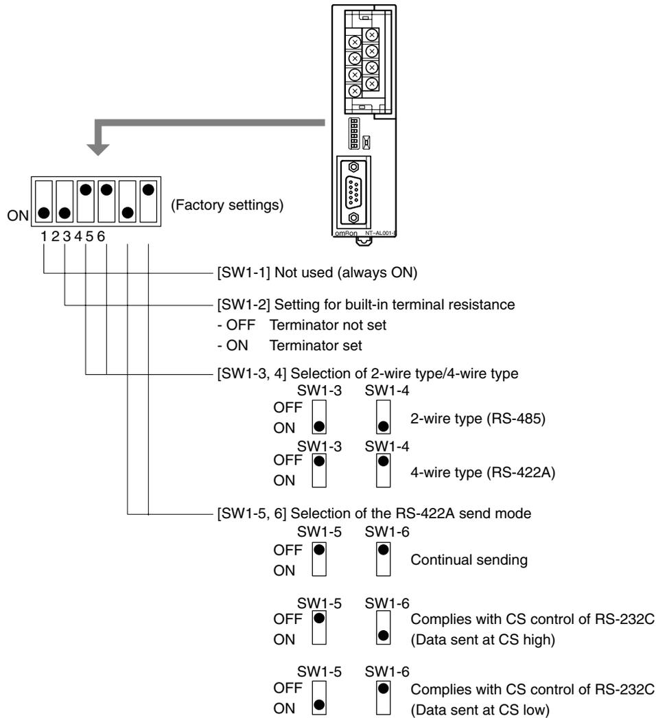
When using the host link or 1:1 NT Link, set the RS-422A send mode to continual sending (set both SW1-5 and 6 OFF).
