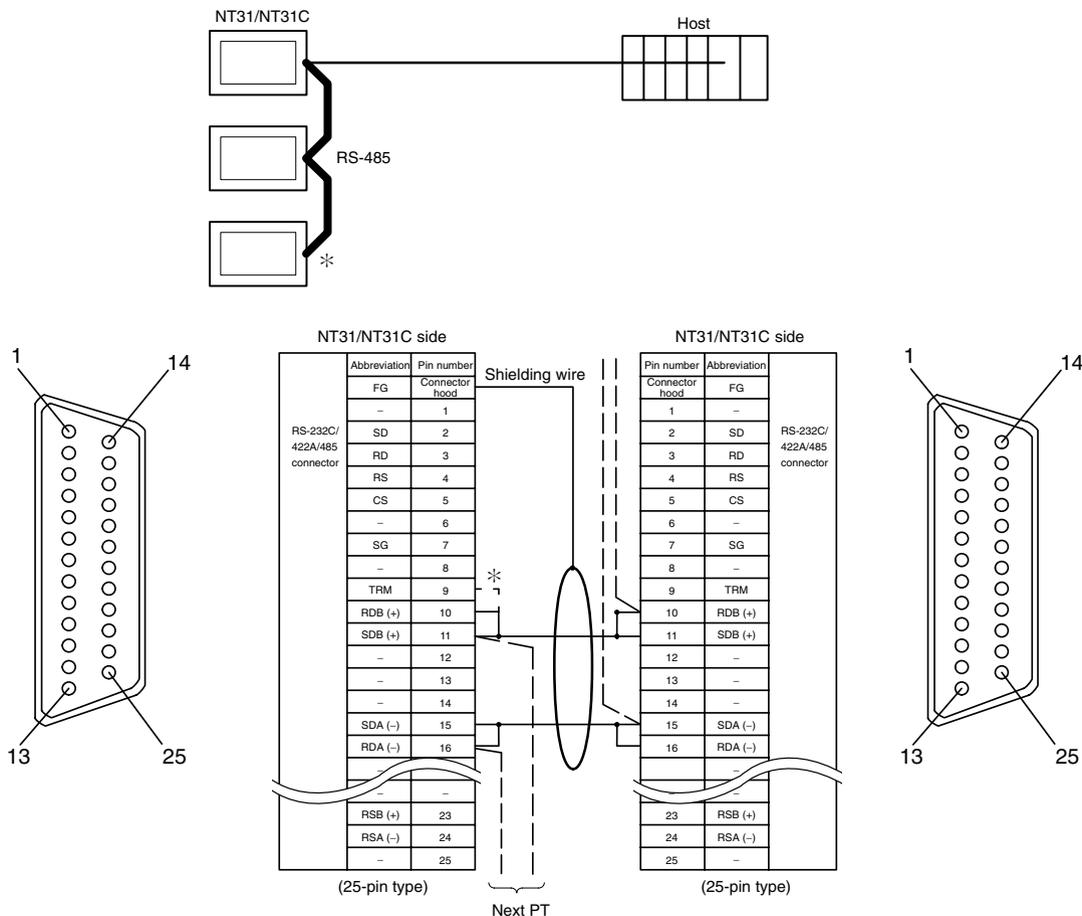
\*2 Make the connection between pin numbers 9 and 10 at the NT31/NT31C at the end of the RS-485 cable (marked \* in the figure above) only.
