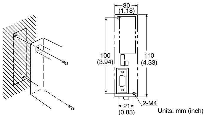
**Note** In order to ensure a secure and strong mount, mount the converter unit in an operation panel with a thickness of at least 2 mm (0.08 inch).
