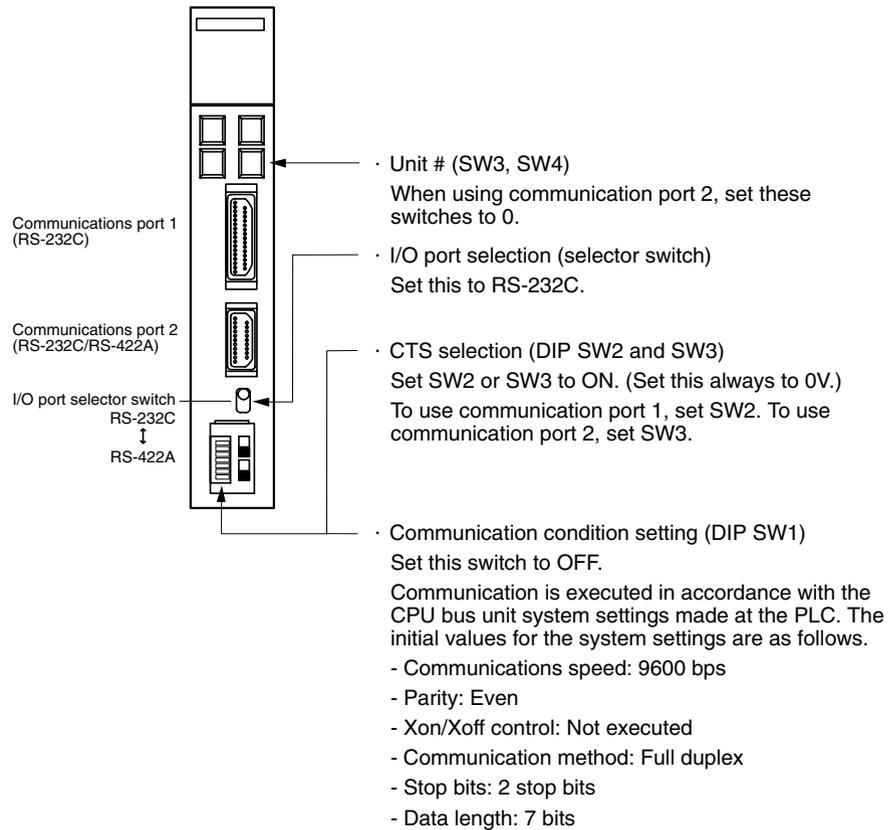
**Connecting to a CS-series Serial Communication Unit**
