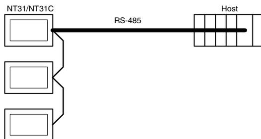
**Wiring When Connecting a CS-series CS1G/H Serial Communication Board, C Series C200HX/HG/HE(-Z)E Communication Board, or CQM1H Serial Communications Board**
