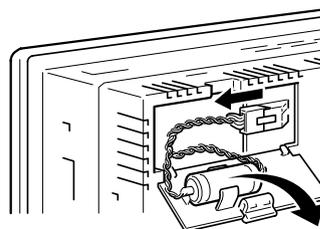
4. Insert the connector of the new battery into the connector on the NT31/NT31C and fit the battery under the battery cover.
