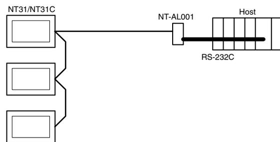
Wiring when connecting a CS-series CS1G/H Serial Communications Board, CQM1H Serial Communications Board, or C-series C200HX/HG/HE(-Z)E Communications Board.
