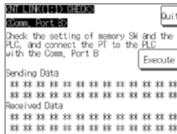
Press Execute to start the check. The data for checking communication is sent to the host, and is displayed as \*\* symbols at Sending Data.
