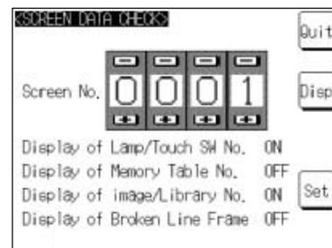
Specify the screen to be displayed in the input field in the middle of the screen.
