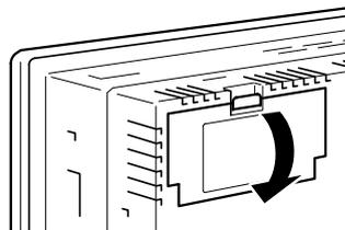
3. Remove the battery that is secured under the battery cover, grip the cable, and pull the connector straight out.
