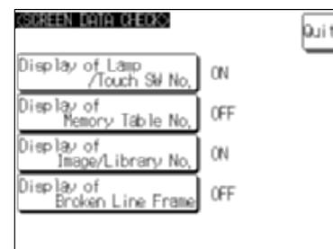
Press the touch switches to specify the display method in each case.
