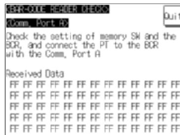
The check starts when the check screen is displayed. Read data with the bar code reader in this status.
