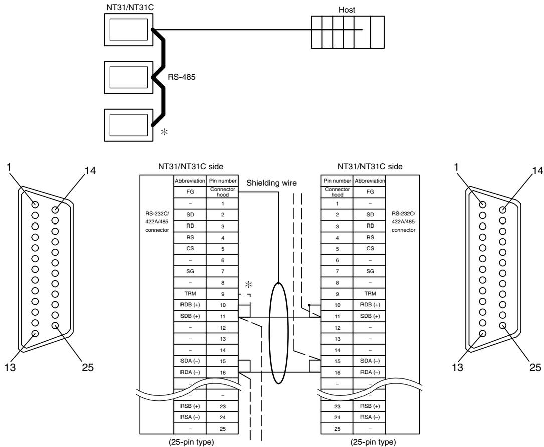
\*2 Make the connection pin numbers 9 and 10 at the terminal NT31/NT31C (marked \* in the figure above).
