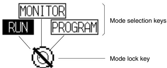
The RUN, MONITOR, and PROGRAM mode selection key elements are touch switches and pressing them causes the PLC operation mode to change (unlike an actual Programming Console, it is possible to switch directly between the RUN mode and the PROGRAM mode.)
