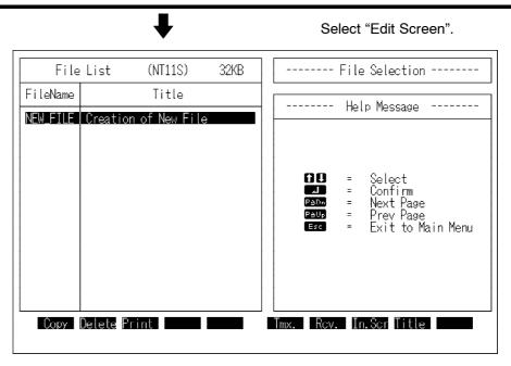
Select a file used for storing the screen data for the NT11S in the "File List" screen.
