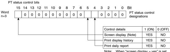
ote: When "screen display = yes" is set, the backlight is lit; when "screen display = no" is set, the backlight is off. NT11S Status Control Section 5-4
