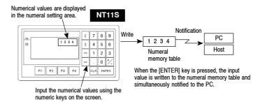
If there is more than one numeral setting area, the one in which the numerical value is to be input can be selected by using  $\boxtimes$ ,  $\boxtimes$ , or  $\boxtimes$  key.
