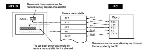
During the operation, the display contents are automatically updated so that the contents of the numeral memory table being displayed are the same as that of the PC word.
