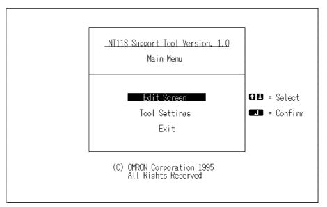
Select "Tool Settings" in the Main Menu to display the "Tool Settings" screen. Settings of Auto Refresh, Communication Port, etc. are made in this screen. Refer to "Setting the support tool for use with the NT11S" on the previous page.
