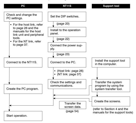
Reference Use support tool NT11S Support Tool (type NT11S-ZA3AT-EV1).
