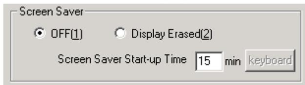
2. When selecting the Display Erased is selected, set the **Screen Saver Start-up Time** to between 1 to 99 minutes. The value can also be input with a keypad that is displayed by clicking the keyboard button.
