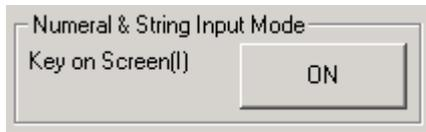
Turn ON the Key on Screen to input numerals and strings with virtual keyboard and keypad.
