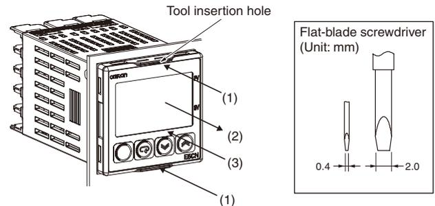
1. Insert a flat-blade screwdriver into the two tool insertion holes (one on the top and one on the bottom) to release the hooks.
