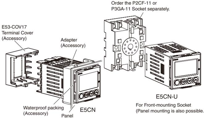
1. The Panel Mounting Adapter is also included with the E5CN-U. There is no waterproof packing included with the E5CN-U.
