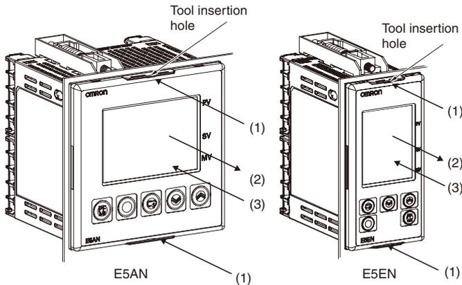
1. Insert a flat-blade screwdriver into the two tool insertion holes (one on the top and one on the bottom) to release the hooks.
