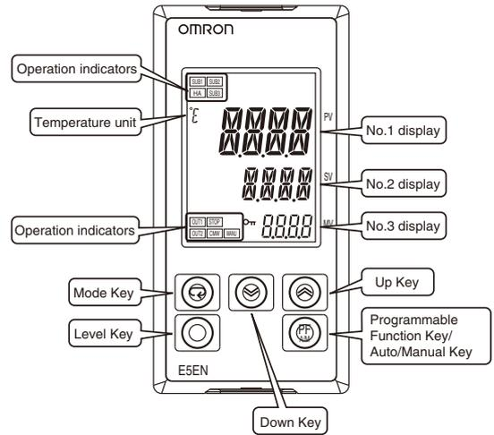
\* A 2-level display when shipped from the factory. A 3-level display is activated if parameters are initialized. For details on the third display level, refer to the *User's Manual, Basic Type* (Cat. No. H156).
