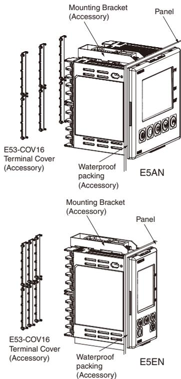
1. Insert the E5AN/E5EN into the square mounting hole in the panel (thickness: 1 to 8 mm). Attach the Mounting Brackets provided with the product to the mounting grooves on the top and bottom surfaces of the rear case.
