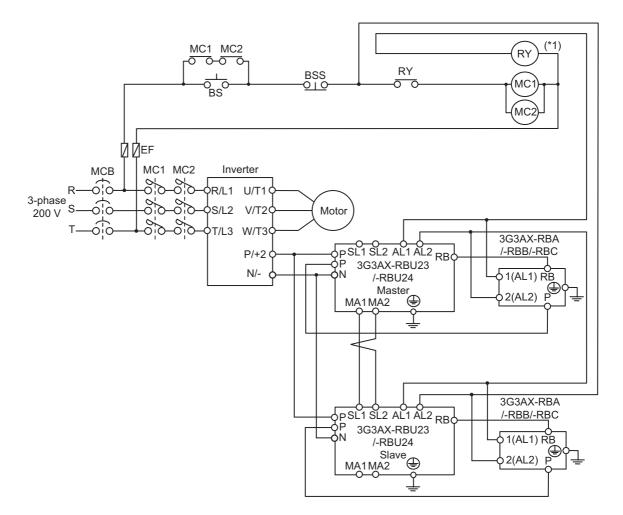
\*1. To select RY, check the MC coil and RY contact specifications.
