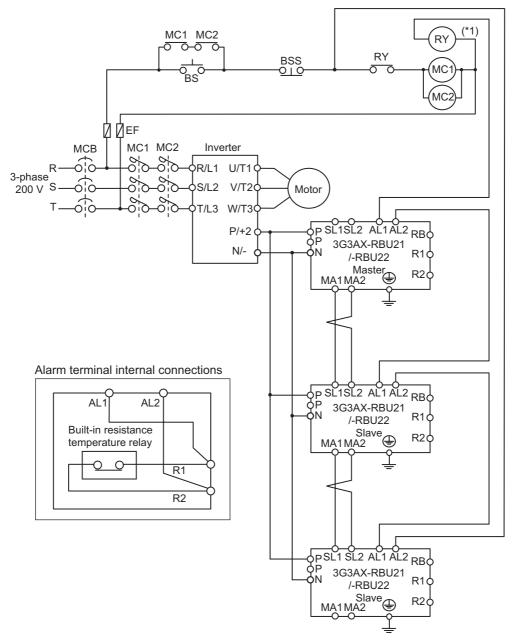
\*1. To select RY, check the MC coil and RY contact specifications.
