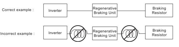
In order to prevent the Braking Register in the Regenerative Braking Unit from burning due to overheating, be sure to connect the alarm contacts (AL1 and AL2) and provide a circuit to turn off the primary power supply for the Inverter.
