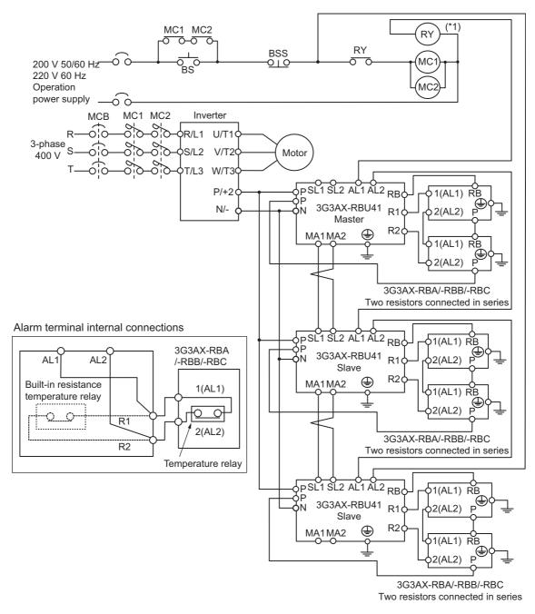
\*1. To select RY, check the MC coil and RY contact specifications.
