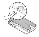
Thread a strap as shown in the picture and tighten it.
