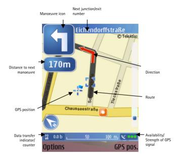
In the turn-by-turn navigation map, the route is displayed in grey. The red arrow shows the direction. The blue arrow shows your GPS position. Turns are displayed in the upper left corner and indicated through voice guidance.
