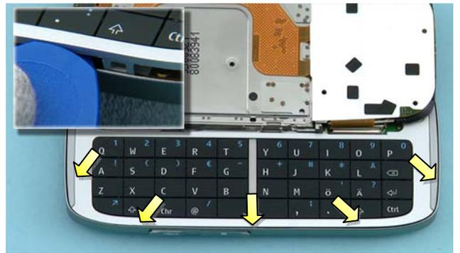
12) Slide the phone open and release the five clips holding the QWERTY KEYMAT using the SRT-6. Release the clip near the space bar first.
