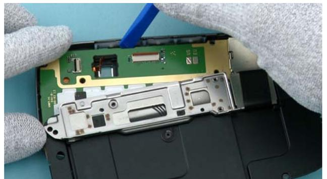
22) Separate the SLIDE MODULE and the engine board from the B-COVER.
