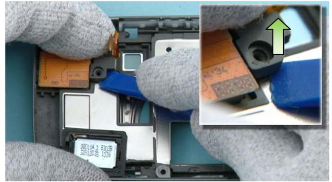
26) To release the AV JACK, slide the SS-93 under the clip and carefully lift it up as shown. Then remove the AV JACK.
