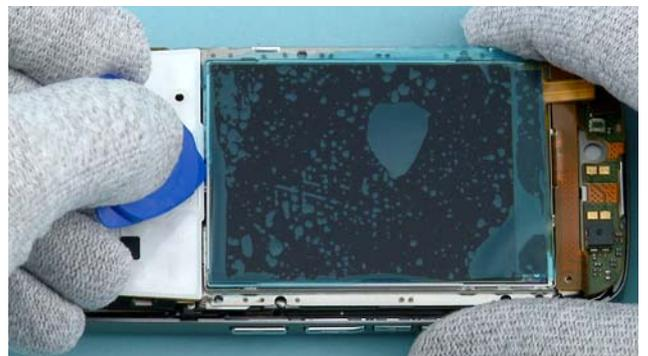
10) Release the LCD with the SRT-6.
