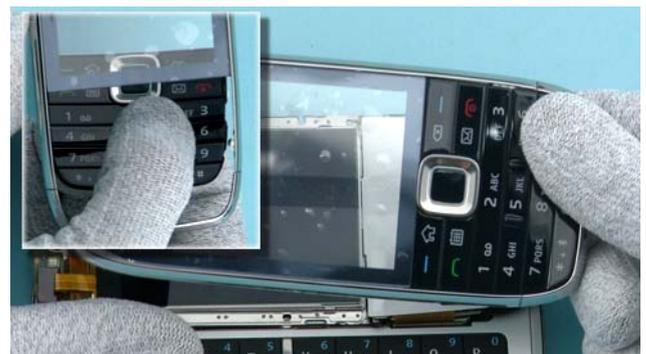
6) Lift up the A-COVER ASSEMBLY. Separate the KEYMAT ASSEMBLY from the A-COVER ASSEMBLY. Remember to protect the LCD with protective film.
