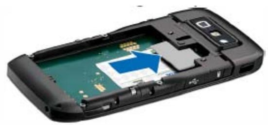
4. Insert the battery. Align the contacts of the battery with the corresponding connectors on the battery compartment and insert in the direction of the arrow.
