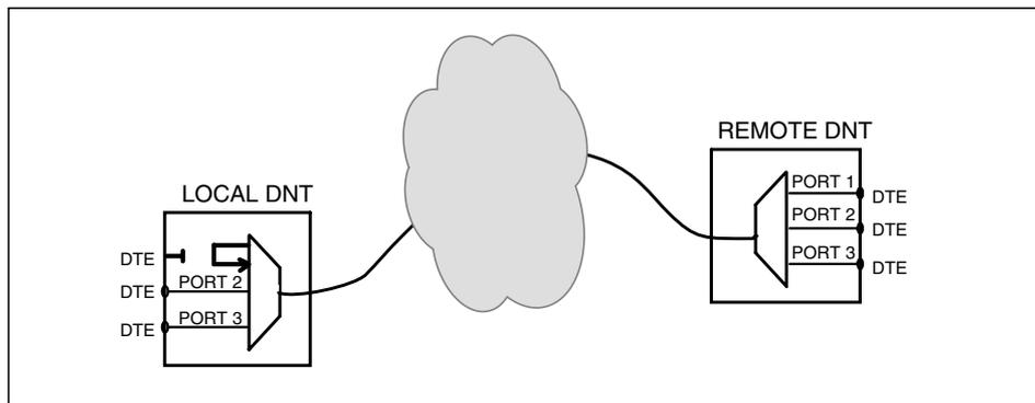
Figure 30. Network test loop (single-port)
