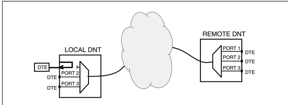
Figure 29. Local test loop in a port
