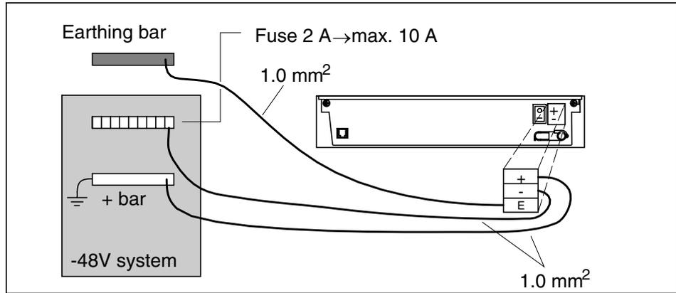
Figure 20. Principle of a negative-grounded DC power system
