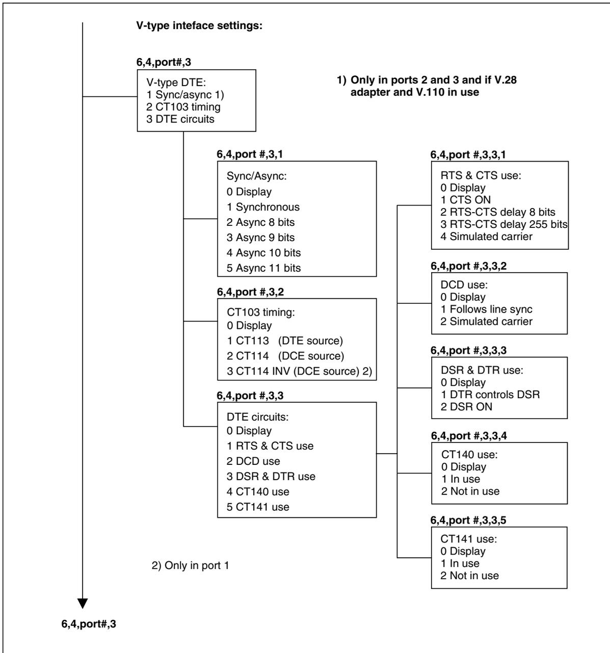
Figure 66. Settings menu structure (continued), V-type adapters
