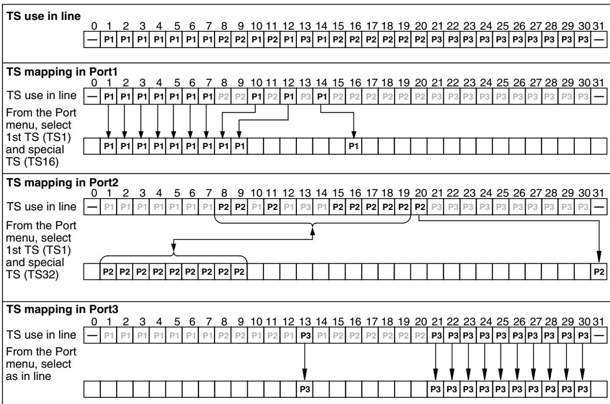
Figure 80. Time slot mapping example, TS0 locally terminated
