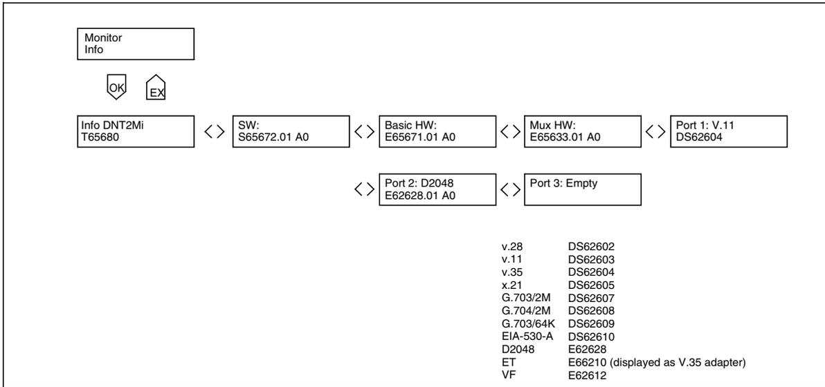
Figure 53. Front panel menus for monitoring equipment information
