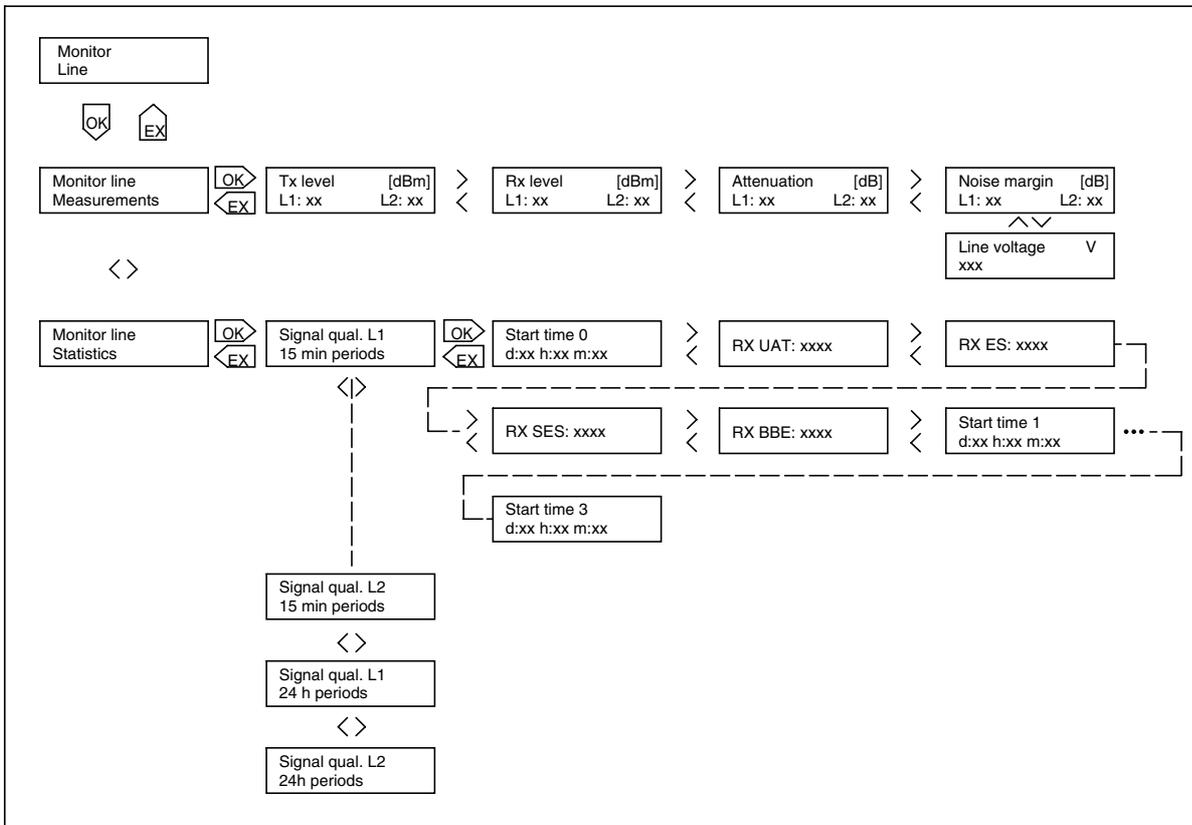
Figure 51. Front panel menus for monitoring a line
