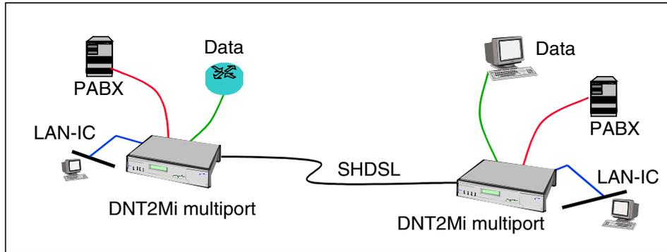
Figure 3. DNT2Mi used in a point-to-point application
