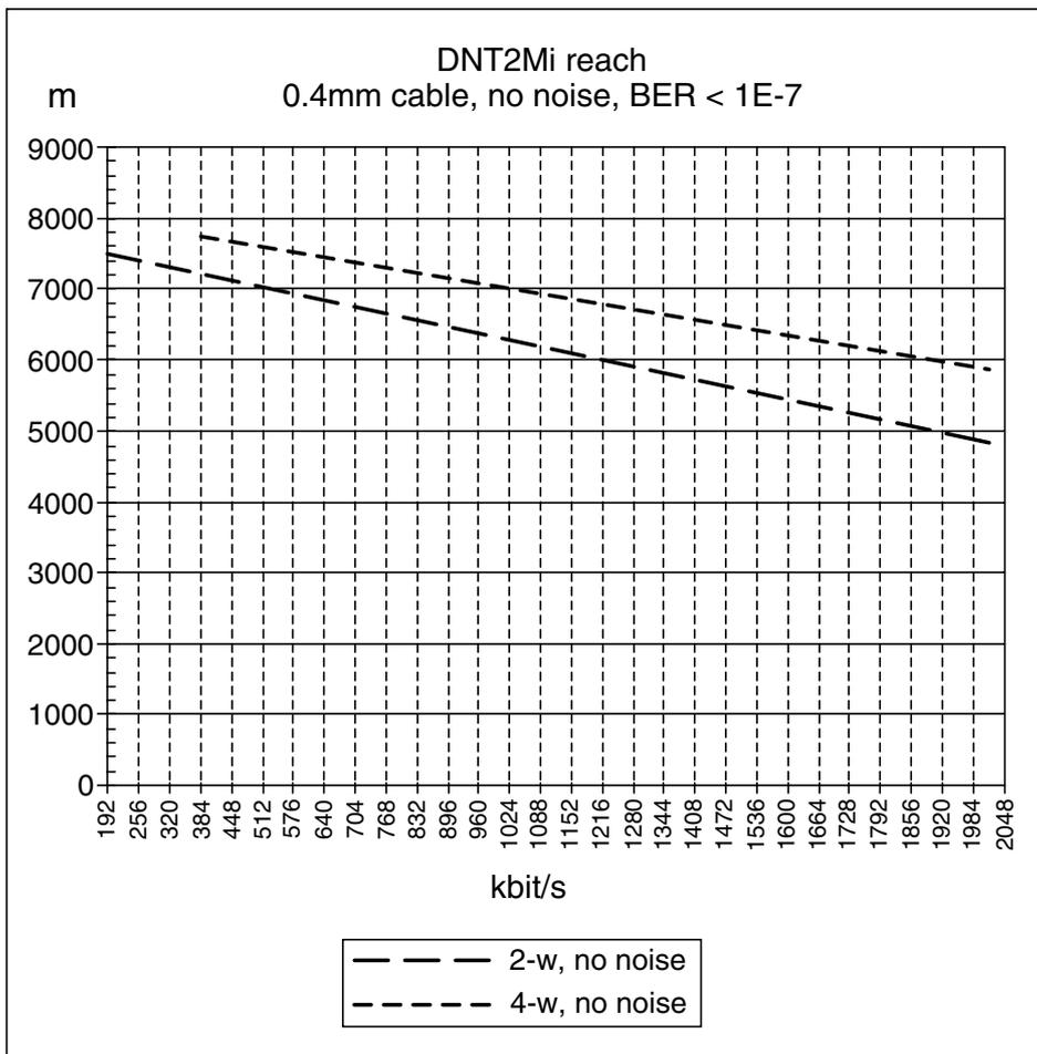
Figure 77. Maximal cable length
