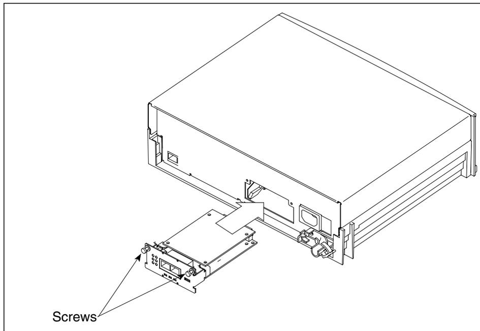
Figure 12. Inserting DTE interface units into DNT2Mi (single-port)
