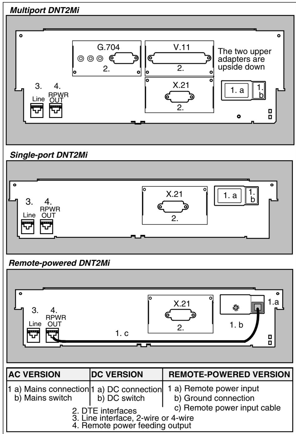
Figure 7. Rear panels of the DNT2Mi units
