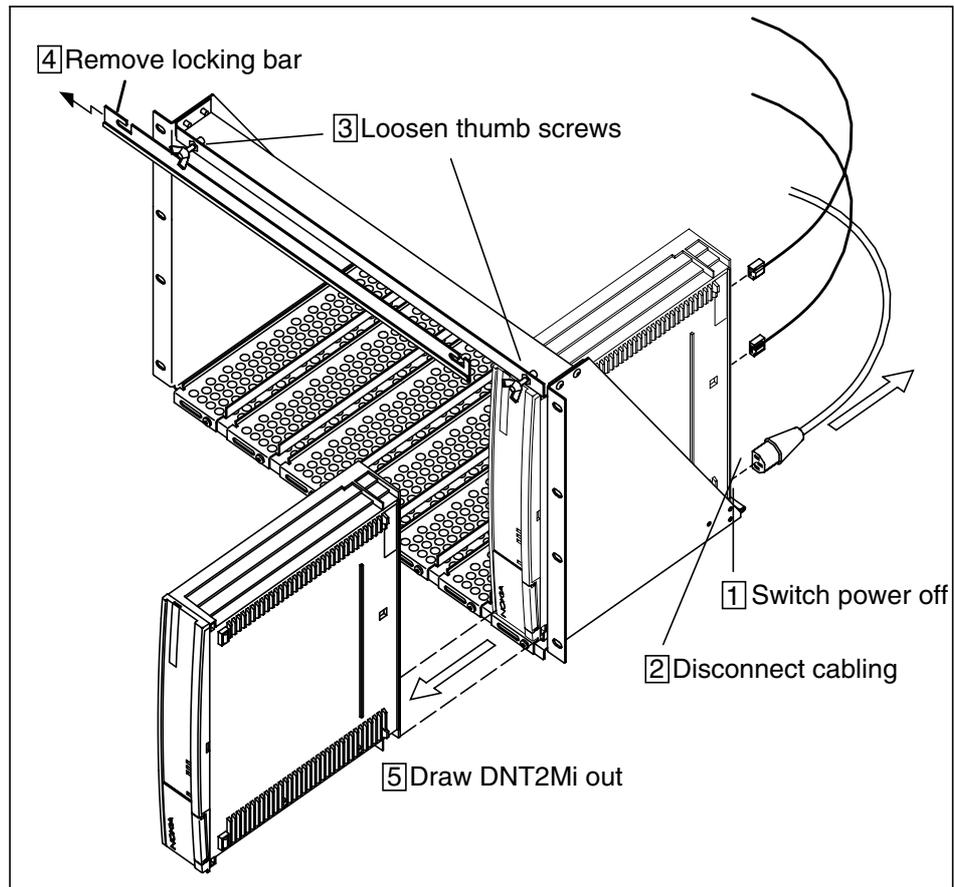
Figure 19. Uninstalling DNT2Mi from a modem shelf
