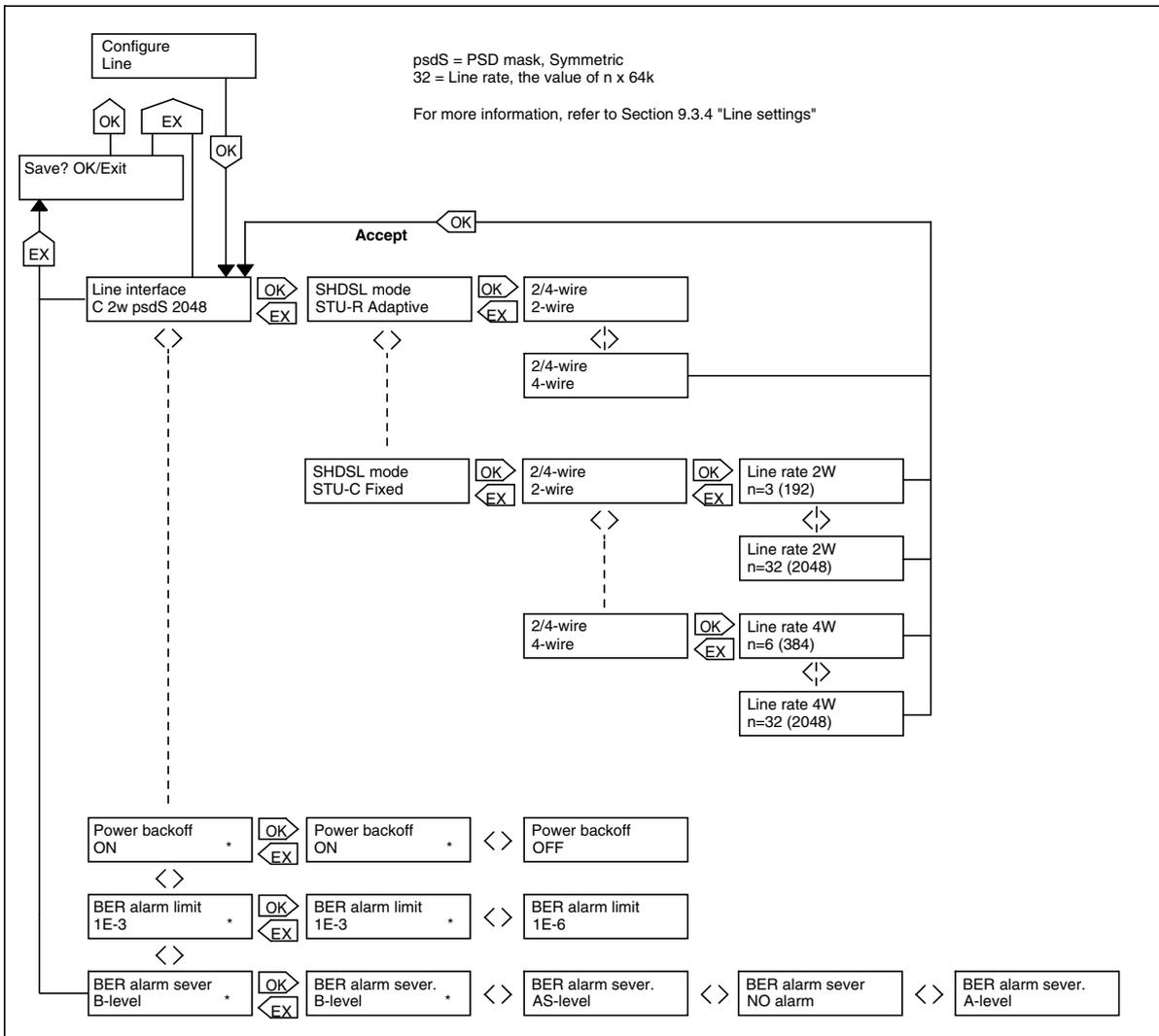
Figure 44. Front panel menus for line settings
