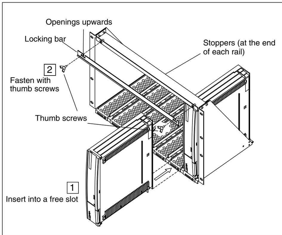
Figure 18. Installation of DNT2Mi in a modem shelf
