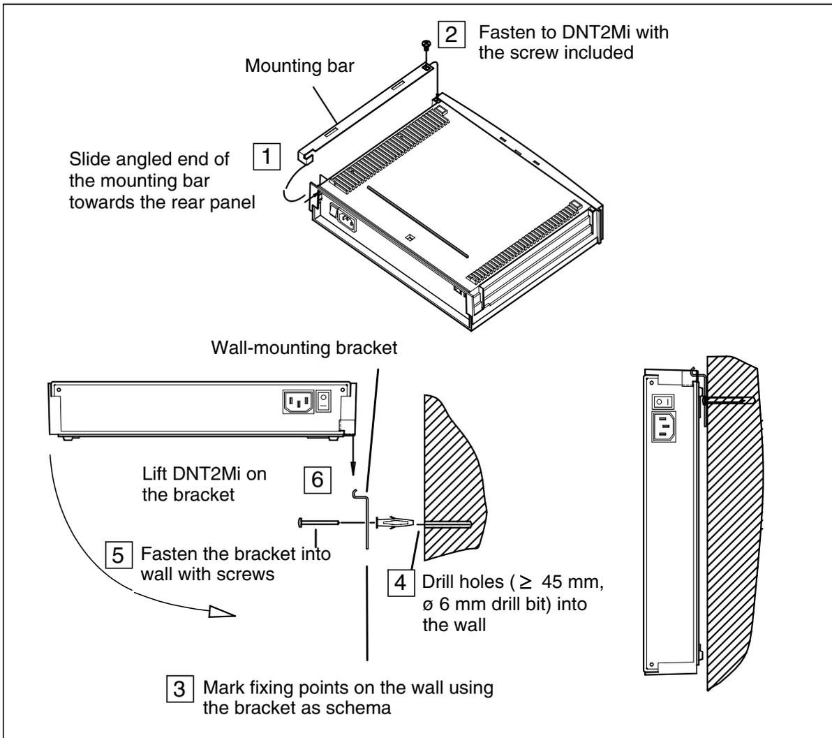
Figure 13. Installation of DNT2Mi on a wall
