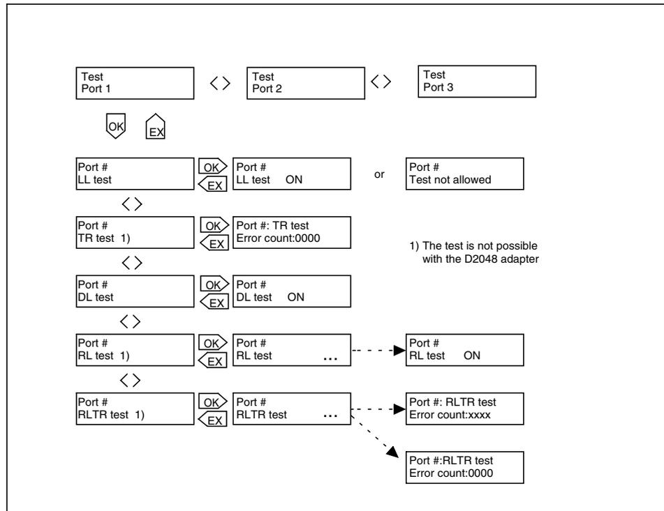
Figure 47. Front panel menus for testing a port
