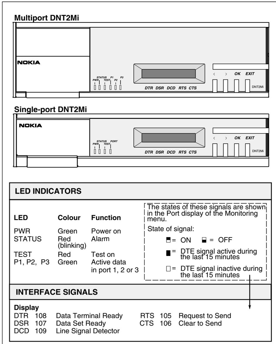
Figure 34. Front panel functions
