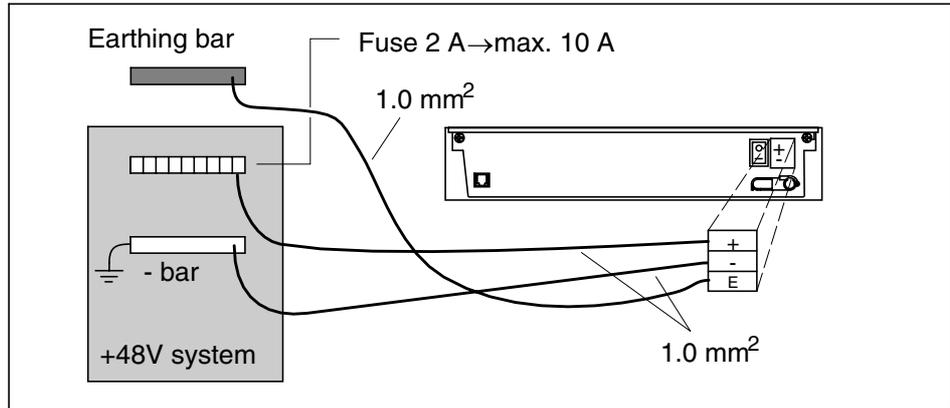
Figure 21. Principle of a positive-grounded DC power system
