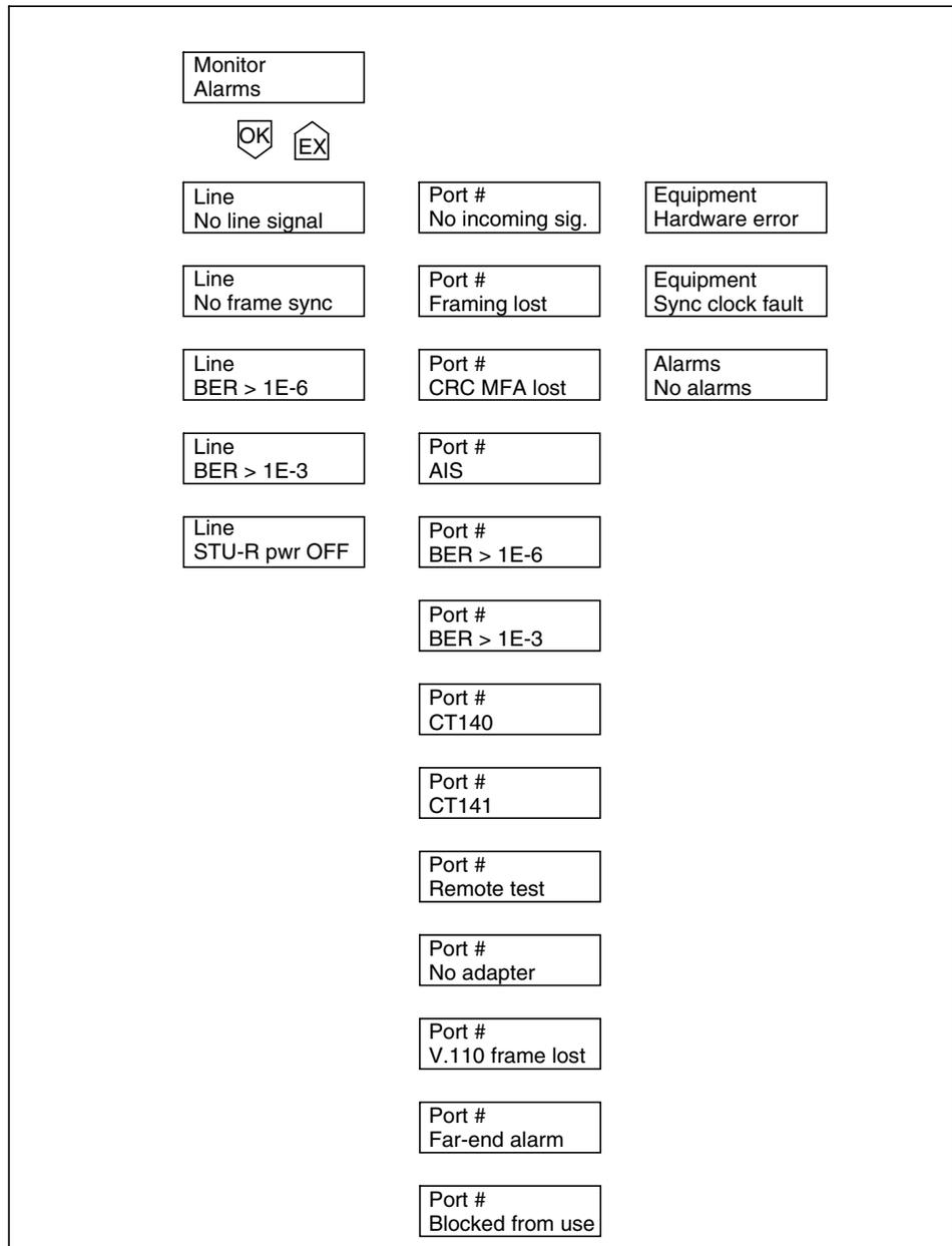
Figure 52. Front panel menus for monitoring alarms
