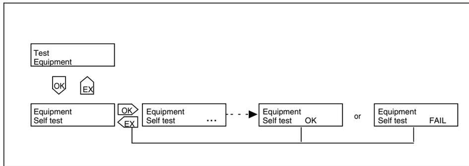
Figure 49. Front panel menus for testing the equipment
