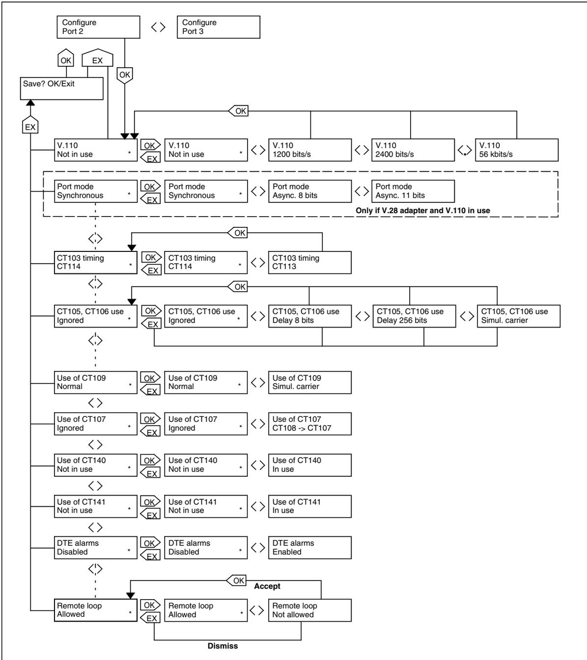
Figure 38. Configuring port 2 and port 3 / V.xx type interfaces
