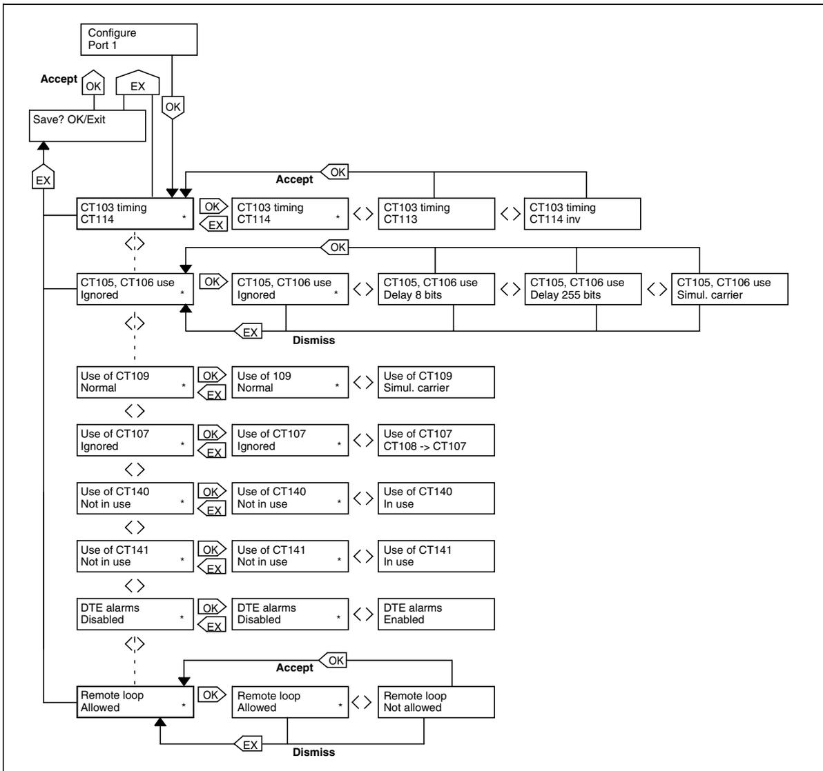
Figure 37. Configuring port 1 / V.xx type interfaces
