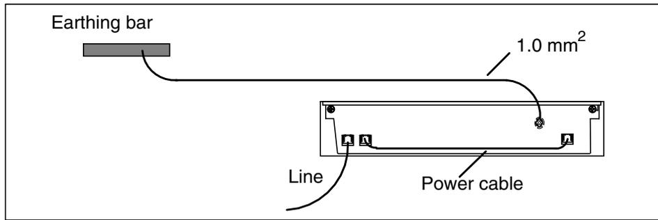
Figure 22. Grounding principle of the remote-powered system
