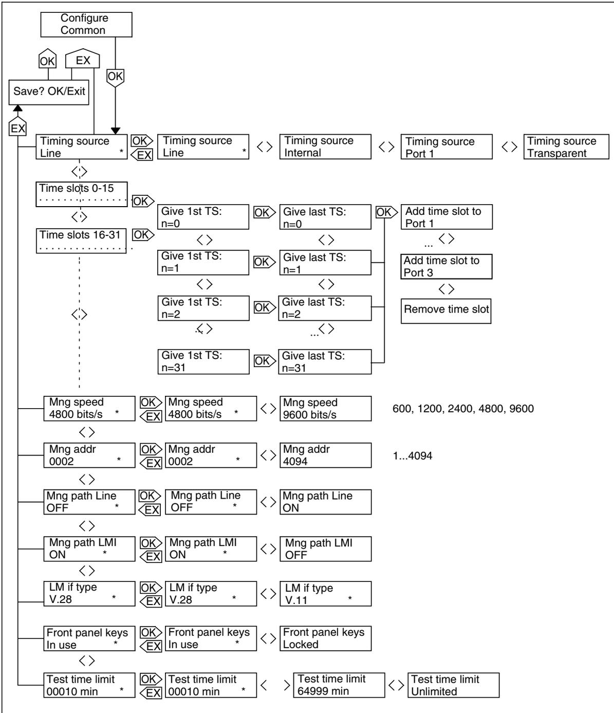
Figure 45. Front panel menus for common settings
