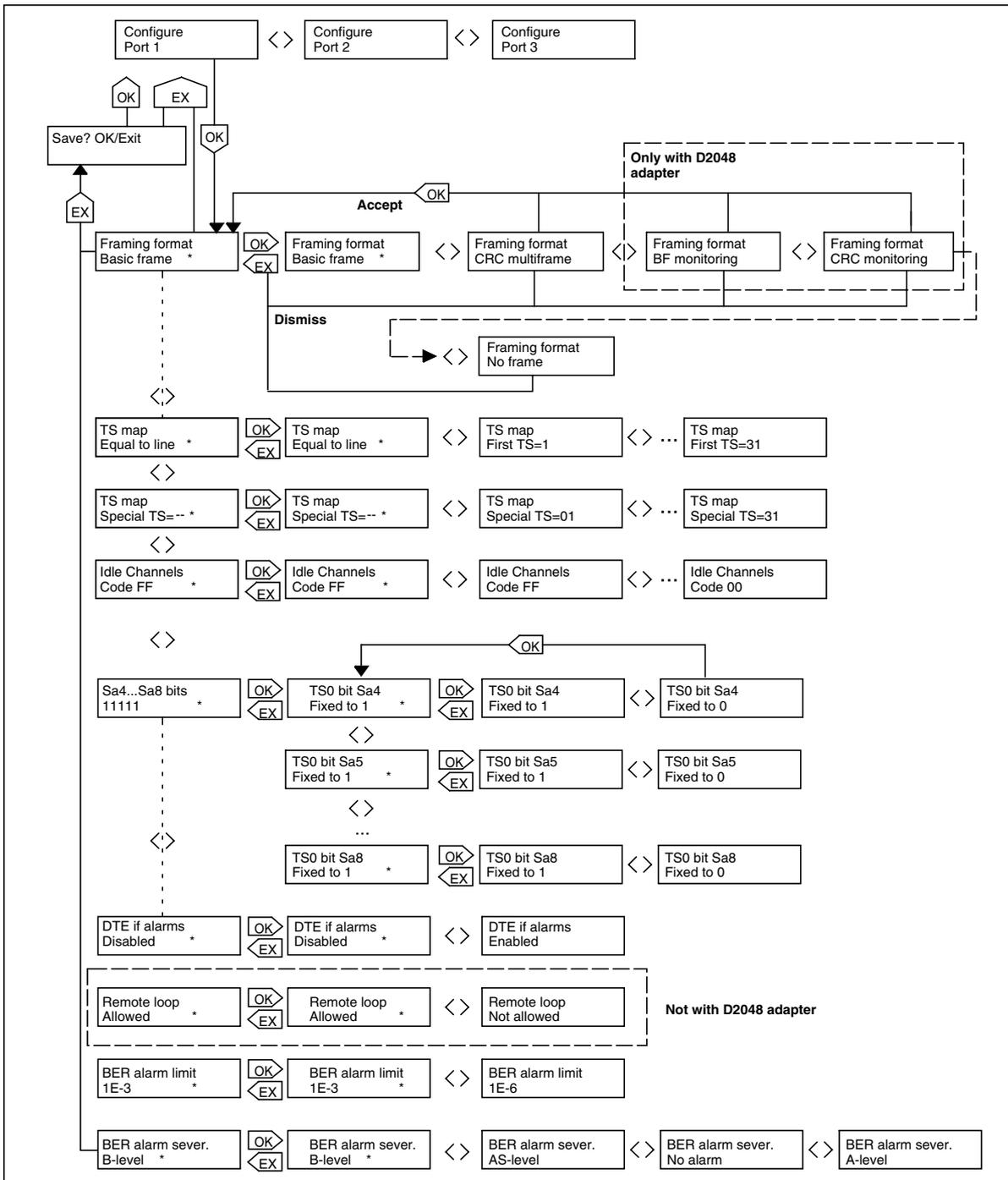
Figure 42. Configuring ports / G.704 interfaces
