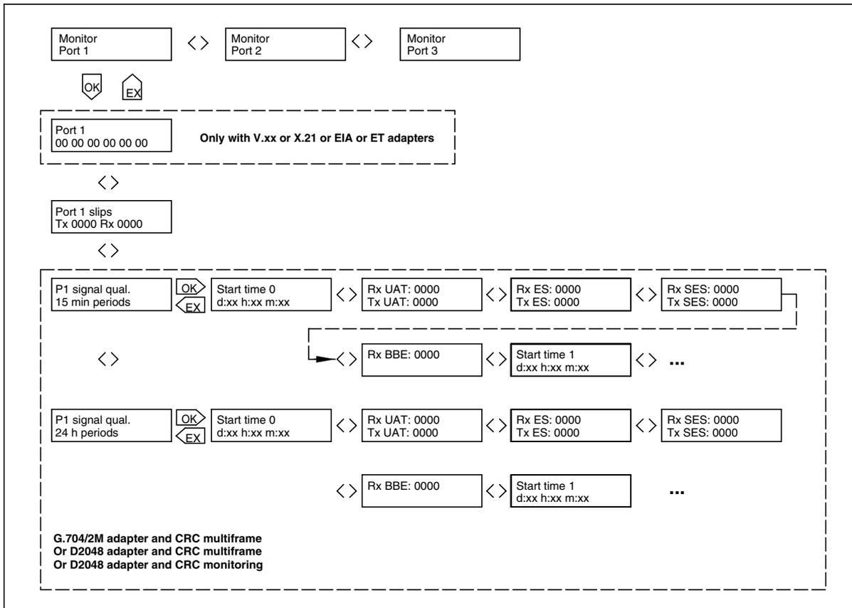
Figure 50. Front panel menus for monitoring a port
