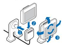
To attach the display to the plate:
