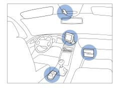
Example of appropriate installation, with the display mounted using the supplied stand
