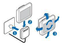
If you need to change the mounting, pull the connector part of the display cable from the ball hinge. To detach the display, pull it from the connector part.
