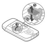
3 Line up the contacts of the battery and the battery compartment, and insert the battery (6). To replace the back cover, direct the bottom locking catches toward their slots (7), and press down until the cover locks into place (8).
