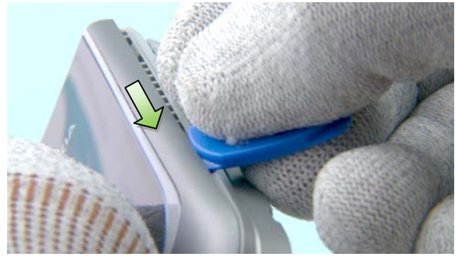
20) Slide the SRT-6 between the A-COVER and the B-COVER as shown.
