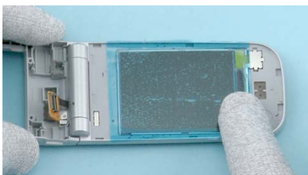
33) Protect the MAIN DISPLAY with protective film.
