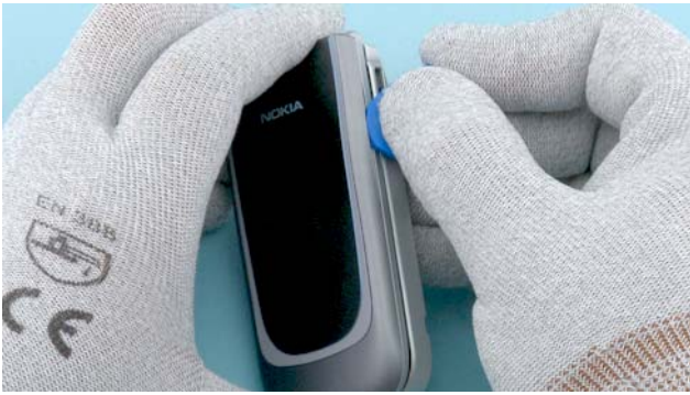
19) Use the SRT-6 to release the A-COVER.
