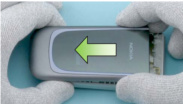
23) Slide the A-COVER to the direction shown to release the final two clips holding the A-COVER. Remove it.
