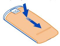
3 Remove the battery, if inserted.
