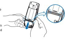
Warning: Use only your hands to remove the battery. Do not use any objects that may damage the phone or the battery.
