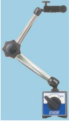
This dial gauge base has an articulated polished aluminium alloy arm, which can be easily locked in any position using the single central locking knob. Plunger and lever indicators are attached using the  $\frac{3}{16}$ in/8mm stem or dovetail fitting system. The arm is mounted on a powerful 80 kilo switchable magnetic base by 8mm x 1.25mm thread. Arm dimensions: lower 110mm, upper 102mm, gauge holder 46mm.
