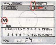
2. Set the SB-24's flash mode selector to A, and the flash sync mode selector to your choice of NORMAL or \* The focal lengths that can be use: RABR
