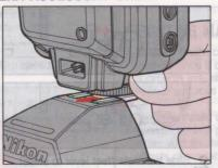
6. Holding the flash near the bottom, slide the mounting foot forward into the camera's accessory shoe as far as it goes.
