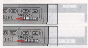
To turn on the speedlight unit, use either STBY (STANDBY) or ON settings. With Nikon F4, F-801/N8008, F-501/N2020, F-401s/N4004s, F-301/N2000, FA, FE2, or FG, to conserve energy, use STBY position.
