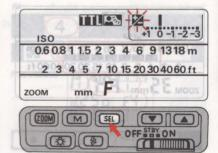
1. Press the SB-24's select button, and confirm the compensation scale appears and ☑ indicator starts blinking in the LCD panel.
