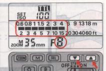
Using the adjustment buttons, select the appropriate aperture to match the shooting distance.
