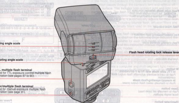
Flash head rotating lock release lever
