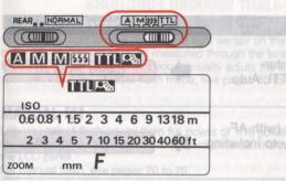
The SB-24's flash mode selector lets you select from four flash modes—TTL Auto . Non-TTL Auto . Manual . or Repeating-Flash . When the power switch is on, the flash mode indicator confirms your selection in the LCD panel.
