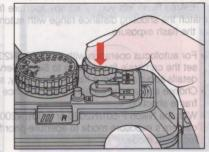
**6.** Fully depress the shutter release button to take the picture.
