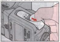
1. Slide the battery chamber cover in the direction of the ▼ and lift to open. Agenty phiaball entine inglity (ma)
