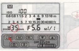
1. Using manual adjustment, set the SB-24's zoom head to correspond to the focal length of the lens you are using.
