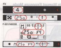
Check the camera's viewfinder to confirm manually selected shutter speed and aperture. The Electronic Analog Display shows the difference in value from the controlled range.
