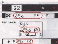
Confirm the controlled aperture and a shutter speed between 1/60 sec. and 1/250 sec. appear in the camera's viewfinder. The aperture-in-use and shooting distance indicator bars appear in the SB-24's LCD panel. With the F-801/N8008, the controlled aperture and shutter speed also appear on the camera's LCD panel.
