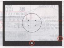
5\_ Lightly press the shutter release button and confirm the ready-light and in-focus matches the shooting distance. indicator are on.
