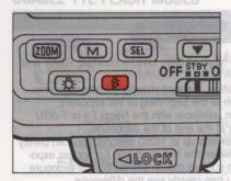
With the SB-24 turned on, its ready-light turns on to indicate the flash is ready to fire. To activate the viewfinder ready-light function when using the Nikon F4, F-801/N8008, F-501/N2020, F-401s/N4004s, F-301/N2000, FA, FE2, or FG, lightly press the shutter release button to turn on the camera's meter.
