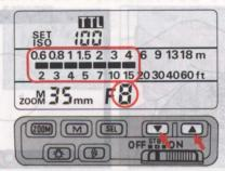
2. Using the adjustment buttons, select the aperture that best matches the shooting distance.
