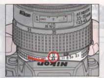
Set lens to minimum aperture (highest f-number). If not properly set, the shutter locks. (F4 shutter displays FEE, but will fire.)
