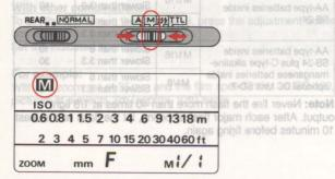
Set the SB-24's flash mode selector to M and the flash sync mode selector to your choise of NORMAL or REAR, then turn on the SB-24.
