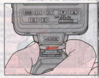
7. Using finger pressure only, gently but firmly tighten the locking wheel.
