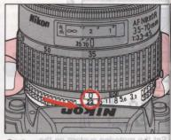
2. Set lens to minimum aperture (i.e. highest f-number). If not properly set, the shutter locks. (F4 shutter displays FEE, but will fire.)
