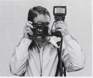
**13.** Take the picture. When the shutter is tripped, the flash unit fires and the picture is taken. Soon, the ready-light will light up to tell you the flash unit is recycled and ready to fire again.
