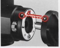
2. Attach the bracket to the flash unit.
