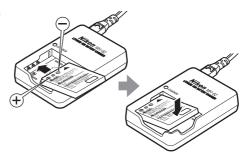
CHARGE lamp starts blinking when battery is inserted. Charging is complete when lamp stops blinking.
