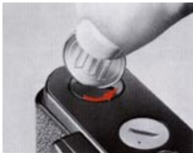
1. Unscrew the camera's motor drive coupling cover.
