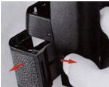
2. Remove the motor drive's battery clip (13).
