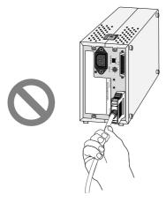
• Do not connect or disconnect the cables while the power is on.
