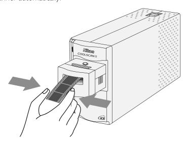
As is the case with mounted slides, strip film should be inserted with the base up and the emulsion surface down. The film is in the correct orientation if the frame numbers on the film are not reversed. The film's edges should be flat or curled slightly downward. Do not use film which curls upwards or which is curled more than 3 mm, as the film may jam or fail to scan properly. Film for use in the scanner should fit in the gauge on top of the adapter.
