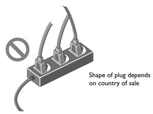
• Use an independent outlet whenever possible. If the scanner is plugged into an outlet to which a household appliance such as a vacuum cleaner or air-conditioner is connected, the scanner's power supply may be subject to noise.
