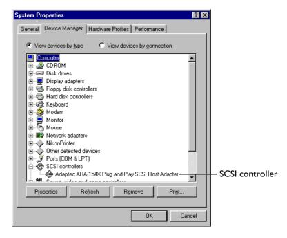
2. If the card has been installed correctly, the System Properties window will contain a "SCSI controllers" icon. If "?" "!" or "X" is showing next to the name of the SCSI adapter, there is a problem which must be resolved before the scanner can be connected. To determine the cause of the problem, select the adapter icon and click the Properties button to view the drivers and system resources for the device.
