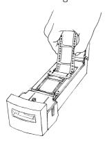
Once the end of the film is free, pull the film slowly backwards out of the adapter with one hand while guiding the free end with the other, being sure that the film does not catch on the adapter or other objects. Keep the angle at which film is pulled from the adapter as low as possible to prevent damage to the film.
