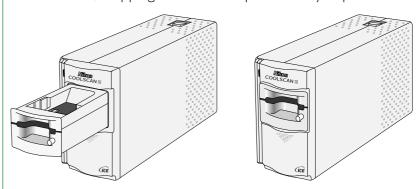
(The illustration above shows the slide adapter. The direction of insertion for other adapters is shown below.)
