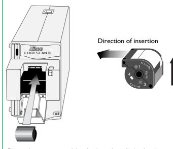
Close the cover, pushing it closed until the latch snaps into place. The scanner will automatically feed film from the IX240 cartridge into the scanner. For details on scanning IX240 film, see the software reference manual.
