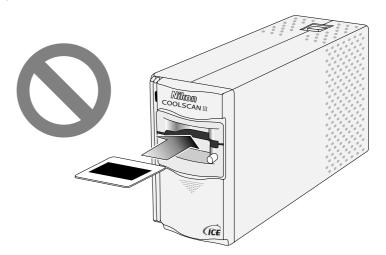
**Note:** The best possible results can be achieved only with clean slides. Before scanning, remove dust from the film with a blower and wipe the slide gently with a soft, dry cloth to remove finger-prints.
