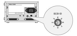
When choosing another ID for the scanner, bear in mind that the computer will usually have an ID of either "0" or "7," and that internal hard disks often have IDs of "0" or "1." In the case of Macintosh computers, the computer will have an ID of "7," while the internal hard disk and CD-ROM drive often have IDs of "0" and "3," respectively. In general, it is recommended that you set the scanner's ID to any number other than zero, one, three, and seven that is not used by another SCSI device.
