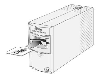
If the scanner is installed on its base, the shiny surface of the film should face to the left and the emulsion surface to the right.
