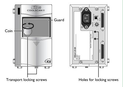
**Caution:** Never turn the scanner on with the locking screws in place. Turning the power on in these circumstances could damage the scanner.
