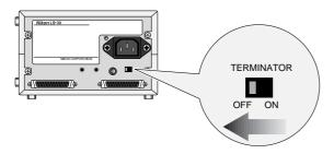
Connect one end of the SCSI cable to either of the connectors on the rear of the scanner, then connect the other end to one of the devices in the chain.
