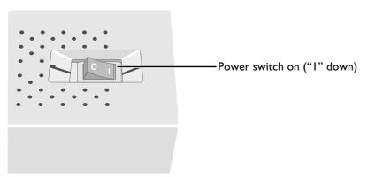
When the scanner is turned on, the status LED will blink while the scanner initializes. Initialization is complete when the LED glows steadily. Once initialization has completed, turn on any other peripheral devices and then start the computer.
