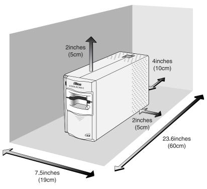
**Caution:** The scanner must be installed with its feet down, as shown in the illustrations on this page. Do not store or operate the scanner in any other orientation.
