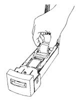
Free the end of the film at the rear of the adapter first by pulling the film upwards a little at a time. Do not pull on the film that remains in the front part of the adapter, as the film could catch in the mechanism and suffer damage.
