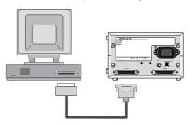
If there are other external devices in the chain, connect the scanner to the last of these devices.
