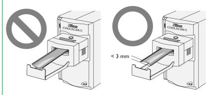
Film will be ejected from the scanner automatically when the scanner is turned on or when no operation is performed for several minutes. Film can also be ejected using the software provided with your scanner. For details of scanning operations, refer to the *User's Guide* or software reference manual.
