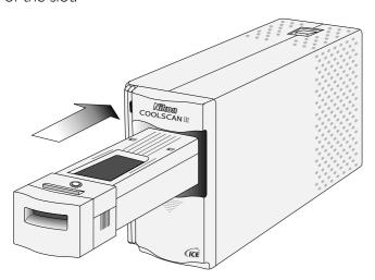
A plastic tray is provided with the strip-film adapter to catch film ejected from the scanner. If the scanner has been installed on its side, this tray can be attached to the adapter by inserting the hooks on the back of the tray into the holes provided on the bottom of the adapter and then pulling the tray slightly forward.
