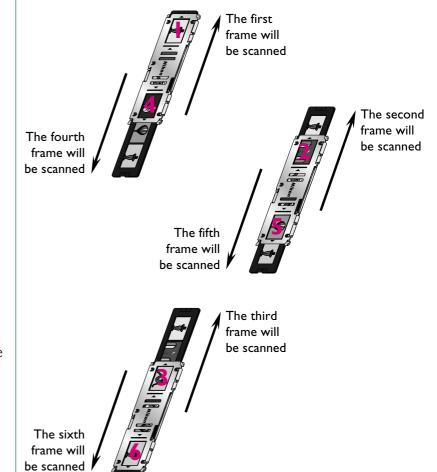
Slide the film holder into the slide adapter until the holder touches the back of the film slot. Do not attempt to force the holder in past the mark.
