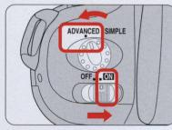
1 Switch power ON and set the camera dial to ADVANCED. The LCD shows the last selected exposure mode/Program. (The original factory setting is for General-Purpose Program.)
