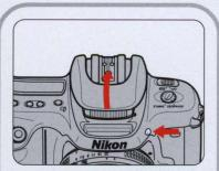
Using Built-In Flash Use the built-in flash not only when the ready-light blinks, but also when your subject is in shadow or backlit. See pages 51 to 55.
