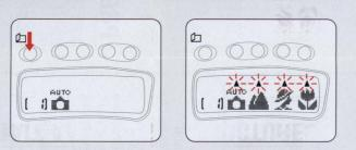
To select the General Purpose Program quickly Just press the menu button for at least two seconds.
