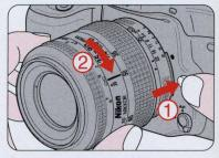
**To remove** While pressing the lens release button, turn the lens clockwise.
