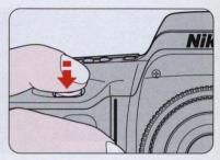
5 Lightly press the shutter release button to activate autofocus operation and the exposure meter.
