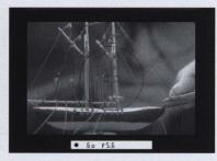
6 Confirm that  $\bullet$  (in-focus indicator), the shutter speed (from 1/2000 to 30 sec.) and an aperture (number with F) appear below the viewfinder screen.
