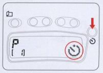
1 Set desired exposure mode or Program, then press the selftimer button. I appears in the LCD panel.
