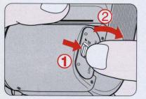
1 Make sure the camera's power is off, then slide the lock release on the battery chamber cover to open the chamber.
