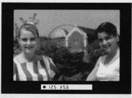
3 While keeping the shutter release button lightly pressed, recompose the picture, then fully depress the shutter release button.
