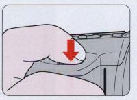
7 Fully depress the shutter release button to take the picture. The film will automatically advance by one frame.
