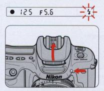
1 When subject brightness is insufficient, the ready-light 4 blinks inside the viewfinder when you lightly press the shutter release button to activate the exposure meter. Press the flash lock-release to release and activate the builtin flash.
