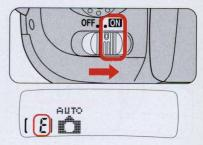
3 Switch the power ON. Check the LCD panel to see if the frame counter shows "E" or the frame number appears and no battery mark ( $\bigcirc$  or  $\bigcirc$ ) appears. If  $\bigcirc$  blinks: Battery is nearing exhaustion. Have a fresh one ready.
