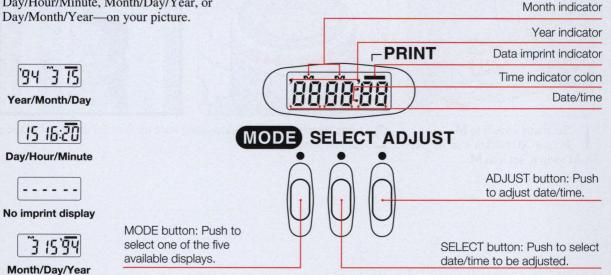
When the LCD becomes faint, replace lithium battery installed in the camera back. (See page 49.)
