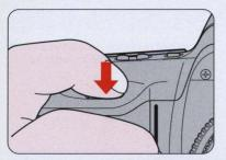
5 Fully depress the shutter release button to take a picture. The film automatically advances by one frame.
