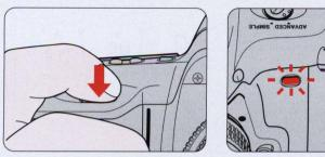
2 Look through the viewfinder, lightly press the shutter release button, and confirm focus and exposure.
