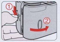
1 Slide the camera back lock release to open the camera back.
