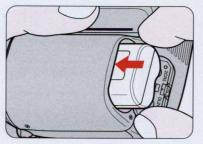
2 Insert a 6V lithium pack with "+" and "-" ends positioned as shown on the inside of the cover. Close the cover by pushing until it clicks.
