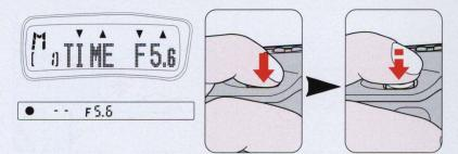
Set exposure mode to Manual and shutter speed to "TIME" (next to "30''") for 30 seconds. Inside the viewfinder, "--" appears in place of the shutter speed indication and the exposure indicator disappears.
