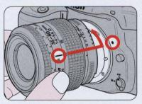
2 Position the lens in the camera's bayonet mount so the mounting indices on the lens and the camera body are aligned. Twist the lens counterclockwise until it locks into place.
