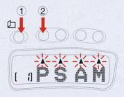
2 Press the menu button (1) to access the exposure mode menu, then press the button above P(2).
