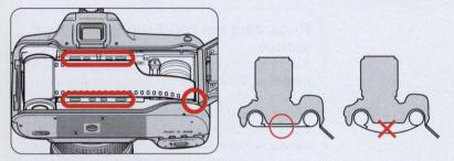
Make sure the film is properly positioned with no slack and the film perforations engage the sprockets. (See illustration.)
