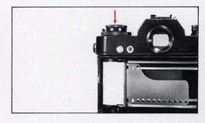
knob and turn it gently in the direction of the arrow until you feel a slight resistance. This takes up any slack in the film cartridge. Then fold back the rewind crank.
