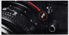
turn the aperture ring until the black needle is in the shutter-speed scale (Take note of the meter's EV range).
