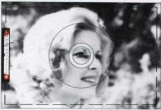
The range surrounded by the broken line is the approximate frame area seen through the viewfinder, and the outer area is the actual printed picture.
