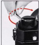
Unfold the rewind crank and turn it with a constant, gentle pressure in the direction of the arrow until you feel an increased tension. Give it a few more turns until the tension has gone and the crank turns freely. The film has now left the take-up spool and the camera may be opened.
