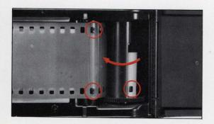
Make two blank exposures to dispose of the first few inches of film which were exposed during loading. When advancing the film, make sure that the rewind knob rotates in the direction opposite the arrow. This indicates that the film has been loaded correctly and is being advanced. The frame counter should now indicate "0" exposure. Advance the film one more frame and you are ready to take the first picture.
