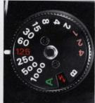
To make manual control, press the shutter speed dial lock in the center of the shutter speed dial, and turn the dial and align the desired shutter speed graduation to the indicator mark. In manual exposure control, intermediate speeds between graduations cannot be used.
